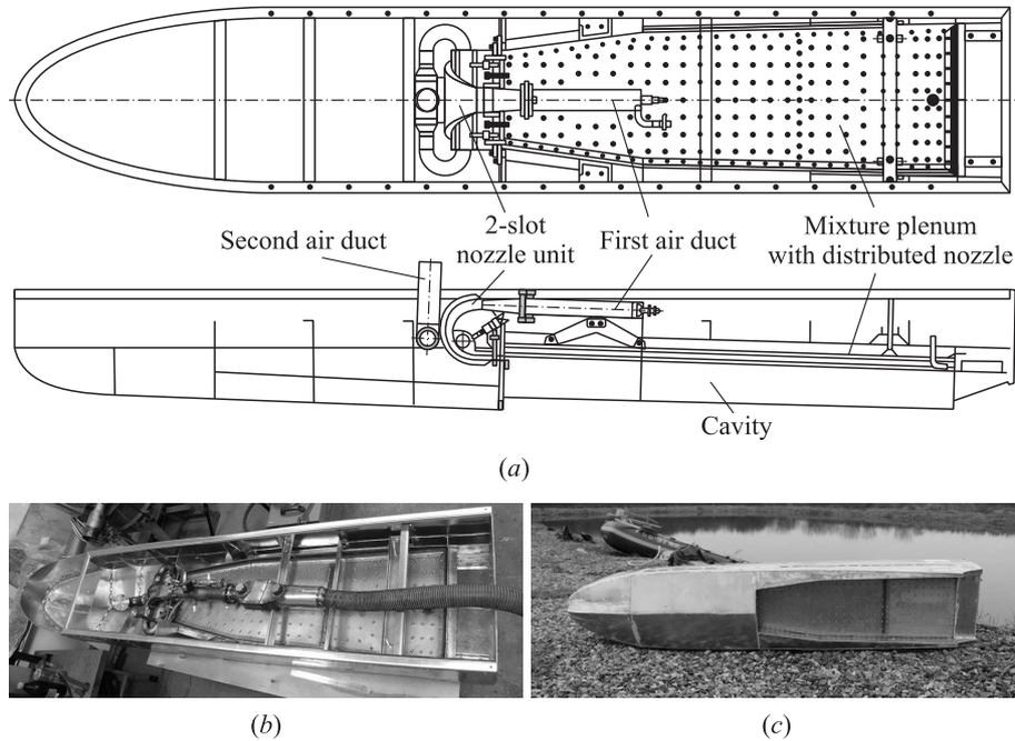
**Figure 2** Schematic (a) and general view (b) of the towed boat and a view of the active gas cavity (c)
