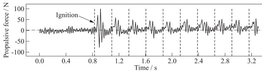
**Figure 8** Primary record of the load cell in the test fire with operation frequency of 3.8 Hz
