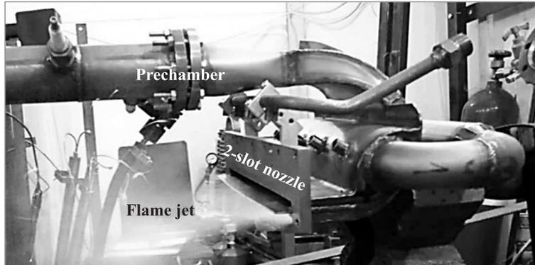
**Figure 3** Imaging of the prechamber flame jet emanating from the lower slot-like opening of the 2-slot nozzle
