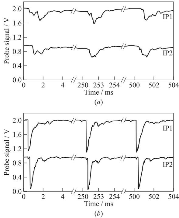
**Figure 4** Records of two ionization probes (IPs) in the prechamber operating in pulsed combustion mode (a) and in pulsed detonation mode (b)
