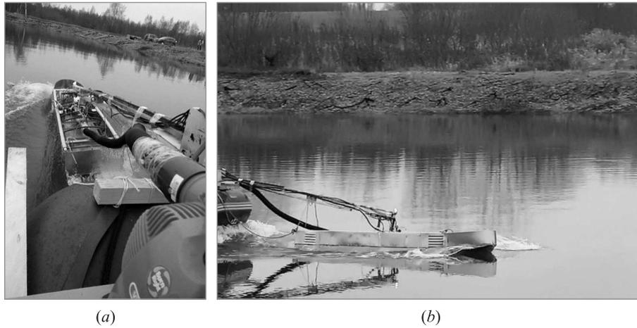
**Figure 7** Video frames of a test fire with pulsed combustion of hydrogen–air mixture in a gas cavity under the bottom of towed boat: (a) filming from the tugboat; and (b) filming from the coast
