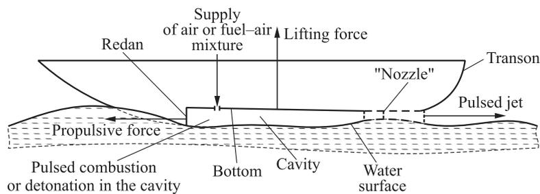
**Figure 1** Schematic of a ship with a bottom gas cavity with stationary / pulsed combustion / detonation of the fuel–air mixture in it
