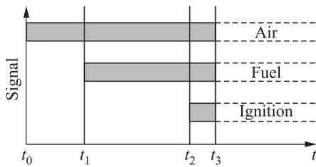
Figure 6 Cyclogram of the operation process in the active gas cavity with pulsed combustion of hydrogen–air mixture
