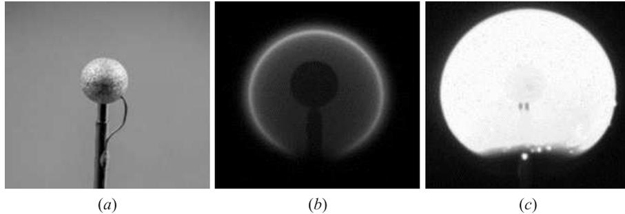
**Figure 1** A PS with a thermocouple and a gas supply tube (a); nonsooting diffusion flame (b); and sooting diffusion flame (c)
