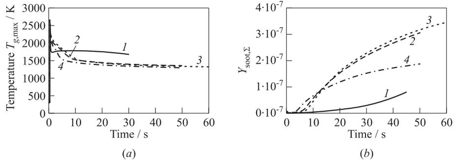
**Figure 5** Predicted time histories of the maximum gas temperature (a) and cumulated soot mass fraction (b): 1 — flame #2; 2 — #8; 3 — #10; and 4 — flame #5
