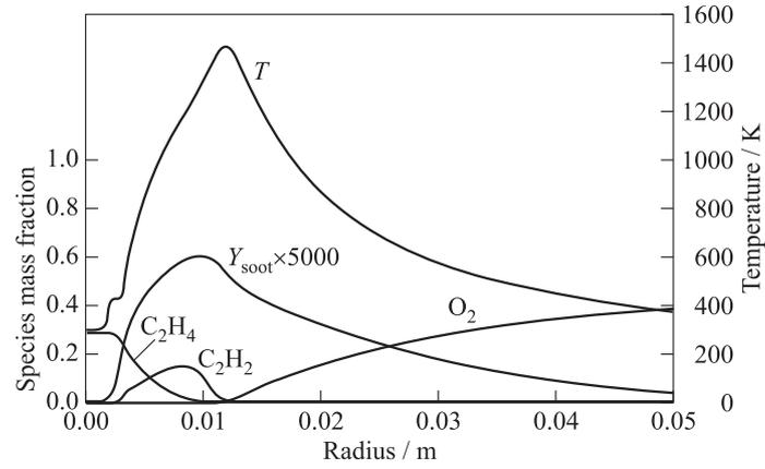
**Figure 6** Spatial distributions of temperature and mass fractions of ethylene, oxygen, acetylene, and soot 20 s after ignition; sooting flame #10
