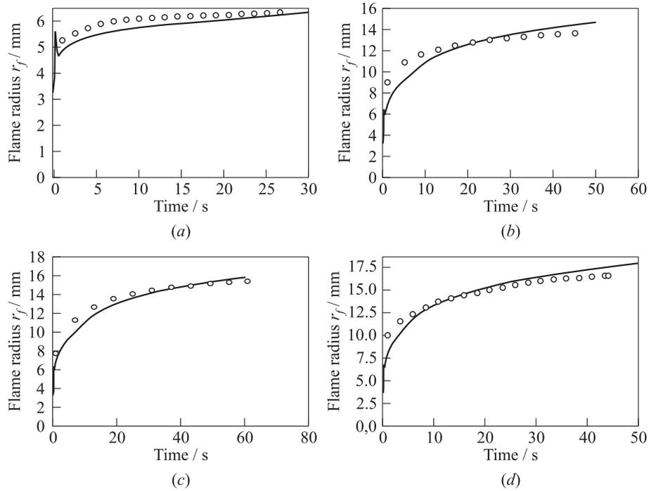
**Figure 3** Comparison of predicted (curves) and measured (signs) time histories of flame radius: (a) flame #2; (b) #8; (c) #10; and (d) flame #5
