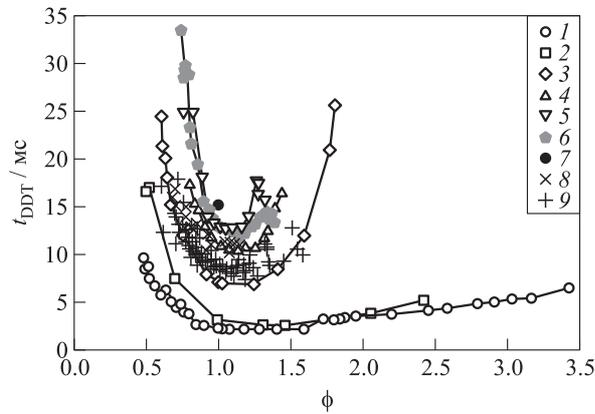
**Figure 8** Dependences of the measured DDT run-up time  $t_{\text{DDT}}$  on the fuel-to-air equivalence ratio  $\phi$  in FAMs of various combustible gases: hydrogen (1), acetylene (2), ethylene (3), propylene (4), propane-butane (5), *n*-pentane (6), NG (7), PP (8), and PE (9)
