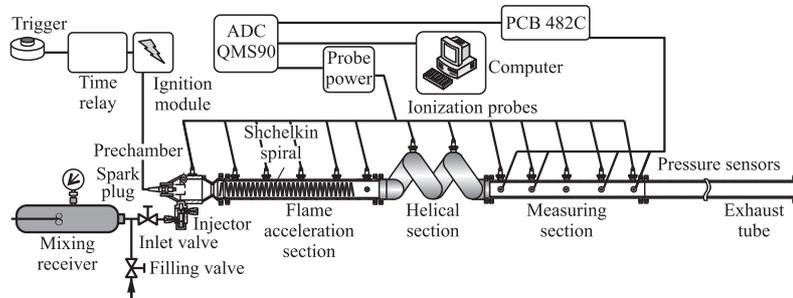
**Figure 1** Schematic of the test bench with the SDT
