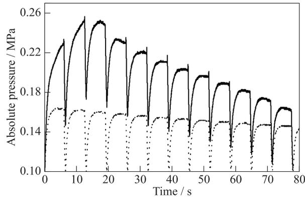
**Figure 4** Typical measured time histories of the absolute pressure in the GG in two tests with 12 shots: in the test with PP sample (solid curve) and in the test without PP sample (dotted curve)
