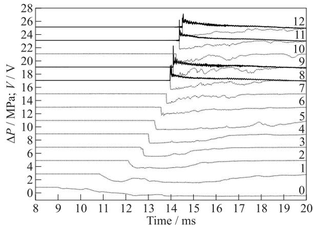
**Figure 5** Primary records of IPs (voltage in volts) in sections 0–12 (dashed curves) and PSs (overpressure in megapascals) in sections 8, 9, 11, and 12 (solid curves) in a test with stoichiometric hydrogen–air mixture
