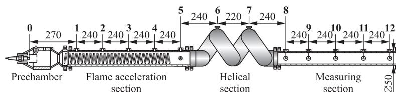
**Figure 2** Schematic of the SDT with the indication of measuring segments: 0 — ignition point; and 1–12 — sections with IPs and/or PSs. Dimensions are in millimeters
