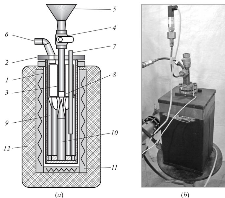
**Figure 3** Gas generator: (a) schematic (1 — casing; 2 — removable cover; 3 — pellet feed tube; 4 — ball valve; 5 — pellet loading hopper; 6 — outlet tube for gaseous pyrolysis products; 7 — thermowell of thermoelectric converter; 8 — protective grill; 9 — metal rods; 10 — metal divider; 11 — muffle furnace; and 12 — thermal insulation); and (b) photograph
