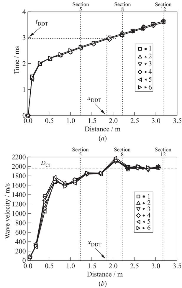
**Figure 6** The distance–time (a) and wave velocity–distance (b) diagrams for six successive shots with the FAMs of the same composition (empty signs — IPs 1 to 6; and filled signs — PSs 1 to 6); a stoichiometric hydrogen–air mixture
