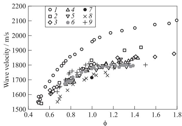
**Figure 7** Measured dependences of the average detonation velocity in the measuring section of the SDT on the fuel-to-air equivalence ratio  $\phi$  for FAMs based on hydrogen  $\text{H}_2$  (1), acetylene  $\text{C}_2\text{H}_2$  (2), ethylene  $\text{C}_2\text{H}_4$  (3), propylene  $\text{C}_3\text{H}_6$  (4), propane-butane  $\text{C}_3\text{H}_8\text{-C}_4\text{H}_{10}$  (5), *n*-pentane  $\text{C}_5\text{H}_{12}$  (6), NG (7), PP (8), and PE (9)
