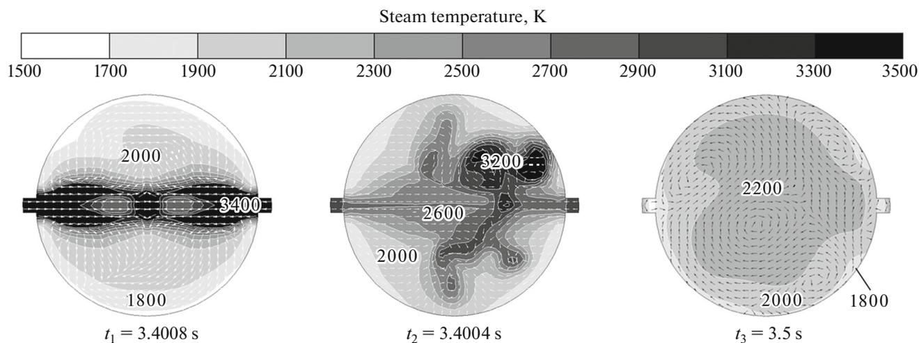
Fig. 2. Calculated HSS flow pattern in the reactor at three times of one detonation shot.
