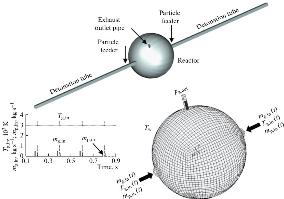
Fig. 1. Schematic, computational mesh, and boundary conditions for a spherical reactor.
