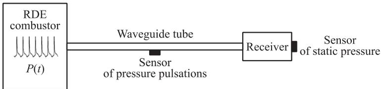
**Figure 1** Schematic of pressure measurements in the RDE using sensors of pressure pulsations and static pressure mounted in a waveguide tube and in a receiver at the tube end-wall;  $P(t)$  stands for the local pressure time history in the RDE
