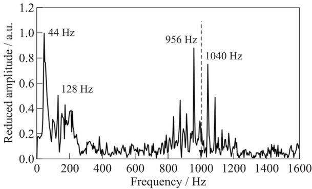
**Figure 3** The FFT of the records of the sensor of pressure pulsations mounted at a lateral wall of a waveguide tube; the frequency of the operation process in RDE is 1000 Hz; the sensor is located in a long waveguide tube 4 mm in diameter at a distance of 0.8 m from the RDE
