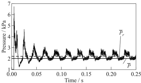
**Figure 2** The calculated records of the static pressure sensor mounted in a receiver at the end-wall of a waveguide tube; receiver volume is  $1 \text{ cm}^3$ ; waveguide tube diameter and length are 4 mm and 2 m, respectively; and the frequency of the operation process in RDE is 1000 Hz:  $\bar{P}$  is the mean static pressure in the RDE; and  $\bar{P}_r$  is the mean static pressure in the receiver
