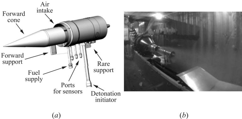
**Figure 1** Hydrogen-fueled CDR: (a) 3D-model; and (b) video frame of CDR test fire in the free-jet wind tunnel before ignition
