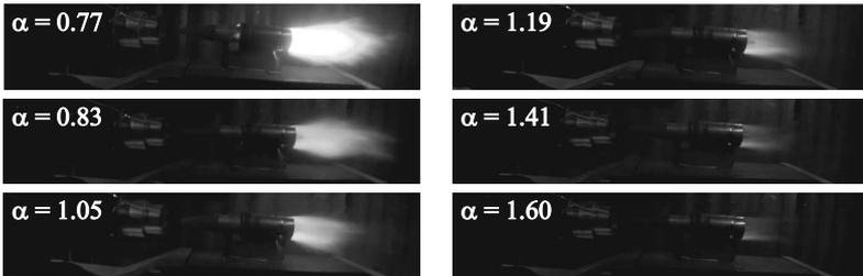
**Figure 2** Video frames of CDR test fires in the free-jet wind tunnel at different  $\alpha$ ;  $M = 1.5$
