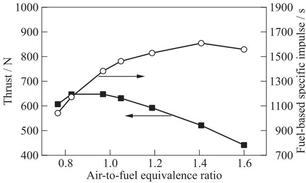
**Figure 3** Measured thrust and specific impulse of the CDR vs. the air-to-fuel equivalence ratio  $\alpha$  in test fires with  $M = 1.5$
