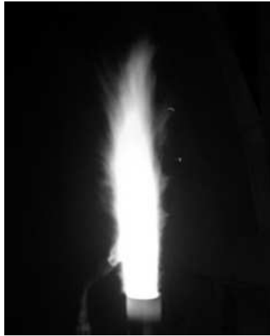
Diffusion flame of the syngas burner during operation
