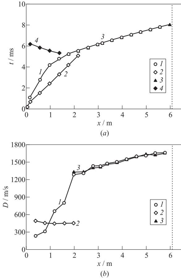
**Figure 7** The space–time diagram (a) and the velocities of the pressure and luminosity fronts (b) for experiment 1 (see Table 4): 1 — luminosity front (flame); 2 — shock front; 3 — detonation front; and 4 — retonation front
