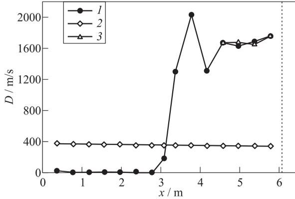
**Figure 5** The velocities of the flame front (1), SW (2), and DW (3) in experiment 5 (see Table 3)
