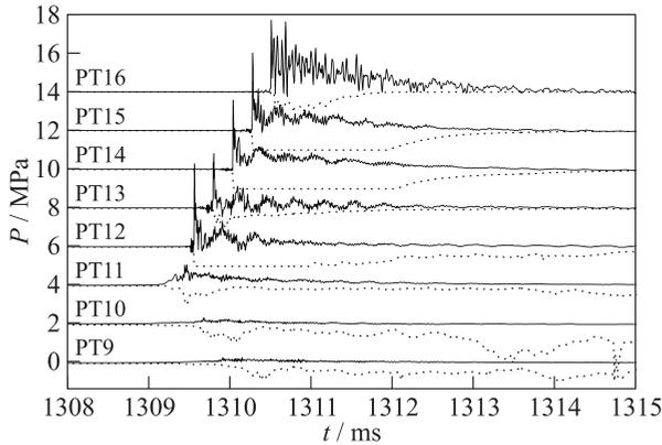
**Figure 4** Records of PTs (solid curves) and PDs (dotted curves) in experiment 5 (see Table 3)
