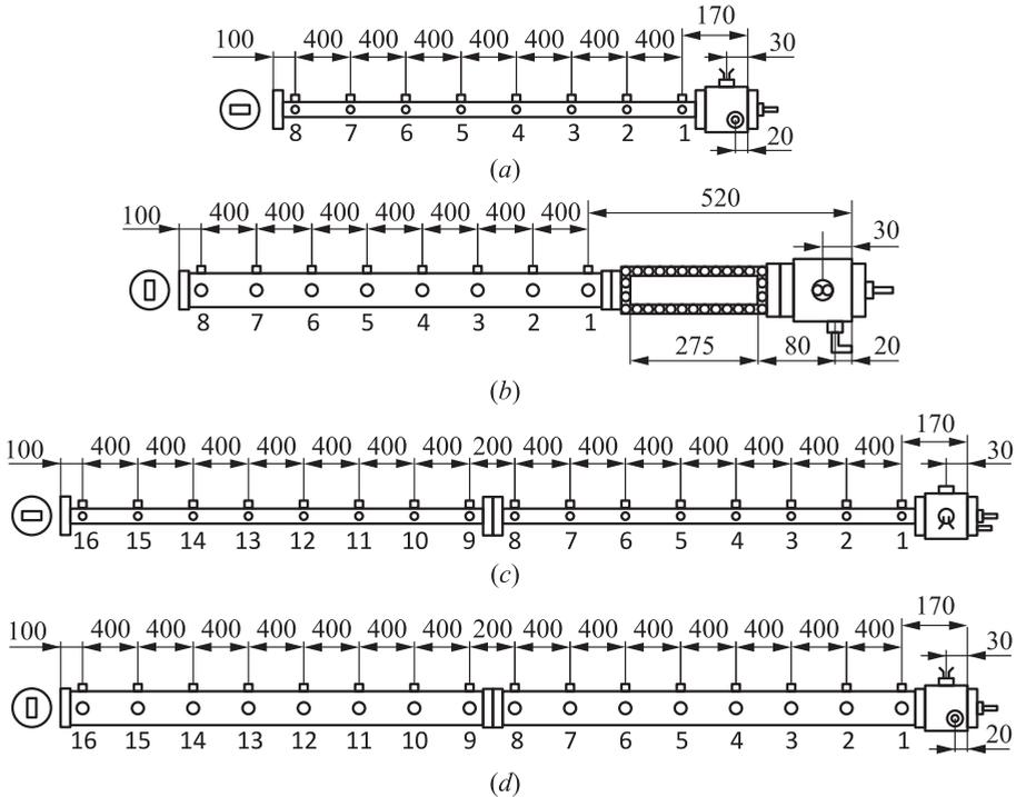
**Figure 1** Schematic of the detonation channel: (a) wide/short channel (height 24 mm, width 54 mm and length 3 m); (b) narrow/short channel (height 54 mm, width 24 mm and 3 m long) with an optical section; (c) wide/long channel (height 24 mm, width 54 mm and length 6 m); and (d) narrow/long channel (height 54 mm, width 24 mm, length 6 m). Dimensions are shown in millimeters
