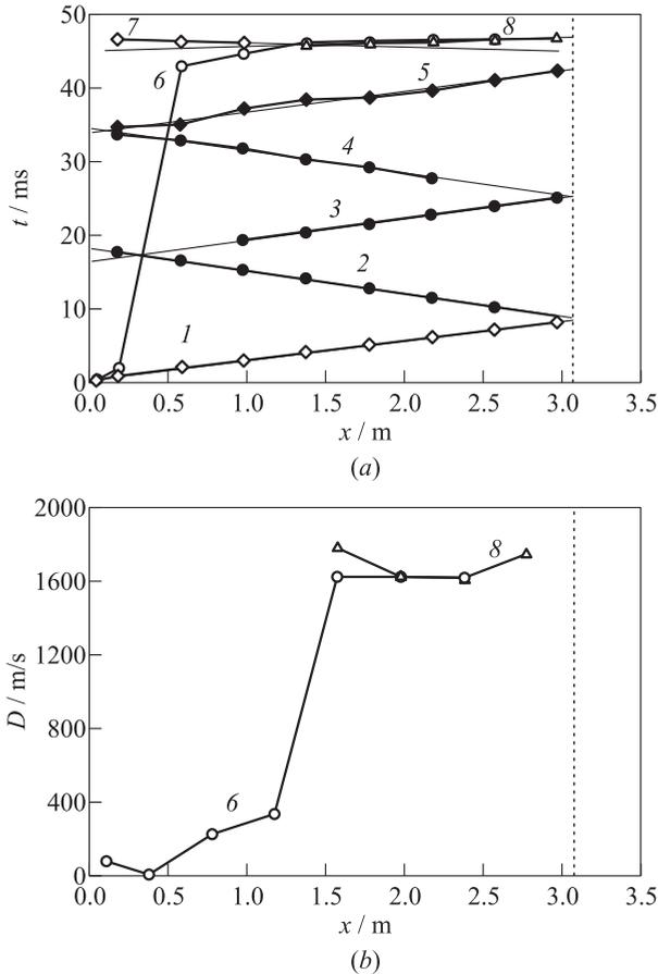
**Figure 3** Space–time diagram (a) and the velocities of the pressure and luminosity fronts (b) for experiment 2 in Table 1: 1 — shock front; 2 — front of the rarefaction wave; 3, 4, and 5 — fronts of acoustic waves; 6 — luminosity front (flame); 7 — front of the retonation wave; and 8 — front of the DW
