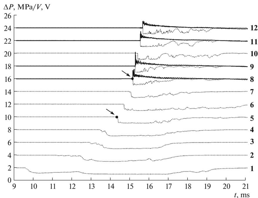
**Fig. 2.** Primary readings of IPs (voltage  $V$ , V) in MSs 1–12 (dashed lines) and PGs (gauge pressure  $\Delta P$ , MPa) in MSs 8, 9, 11, and 12 (solid lines) in a single shot in an experiment with an FAM based on the products of the PG pyrolysis at a decomposition temperature of 700°C.
