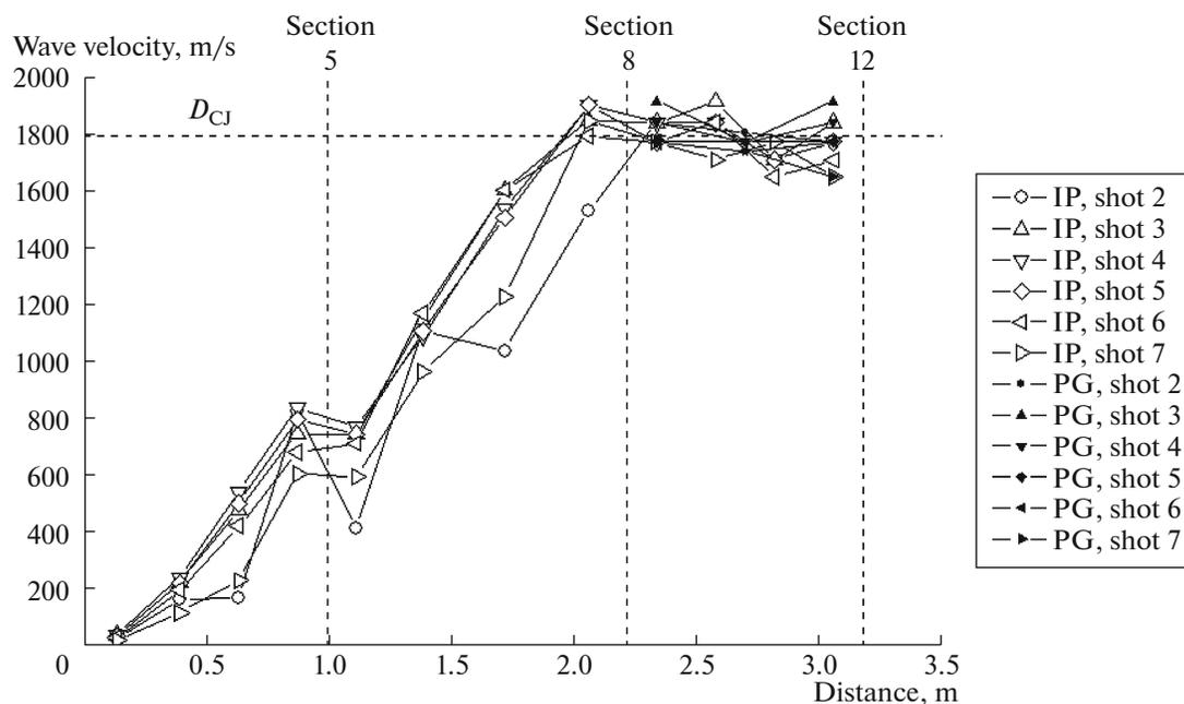
**Fig. 3.** Dependences of the velocities of the flame front and the pressure wave on the travelled distance in six successive shots 2–7 in experiment 40 with an FAM based on PGPP.
