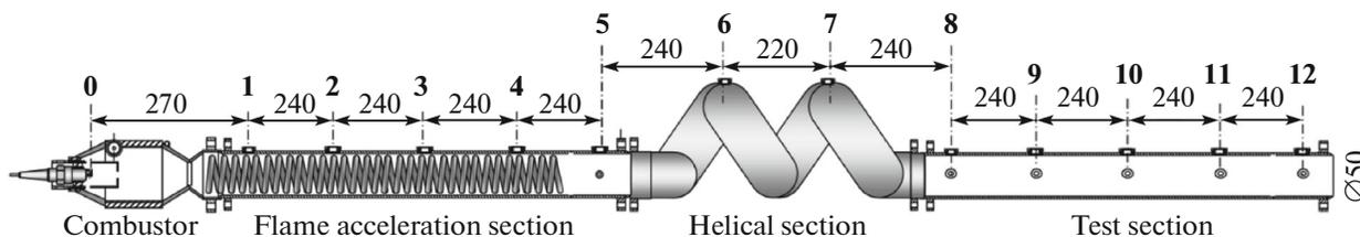
**Fig. 1.** Scheme of the calibration pulsed-detonation wind tunnel, including base distances (in mm): 0, ignition site; 1–12, measurement sections, in which PIs and/or PGs are installed.
