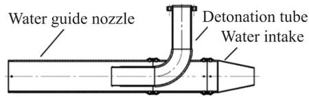
**Figure 1** Schematic of the PDH
