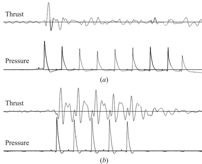
**Figure 3** Thrust and in-chamber pressure records at deactivated (a) and activated (b) exhaust valve at PDH operation with 14 Hz
