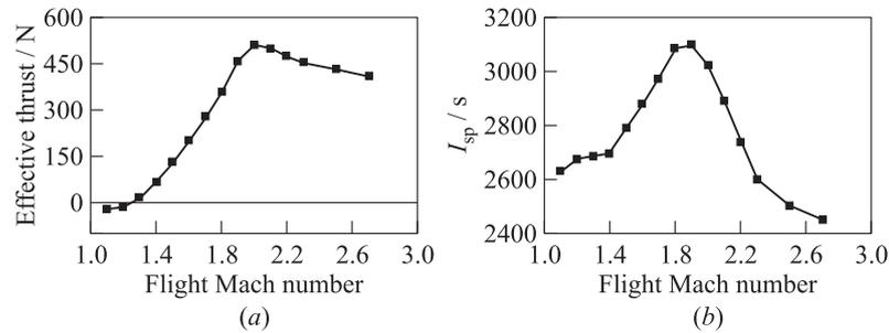
**Figure 2** Calculated dependencies of the effective thrust (a) and fuel-based specific impulse (b) on the flight Mach number
