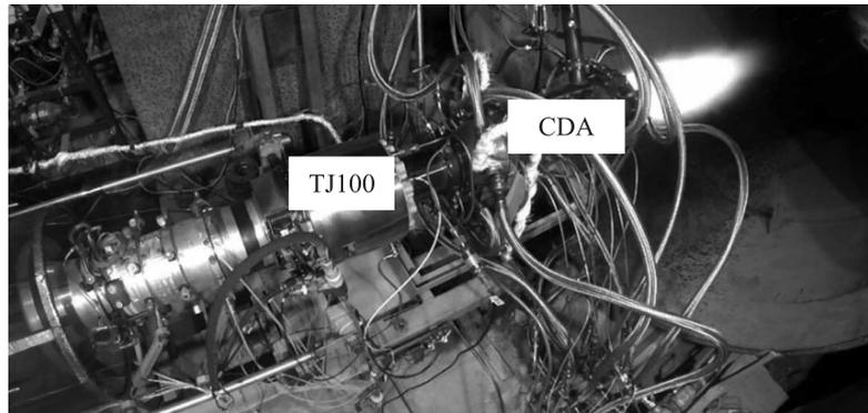
**Figure 1** Test rig with TJ100–CDA assembly during firing
