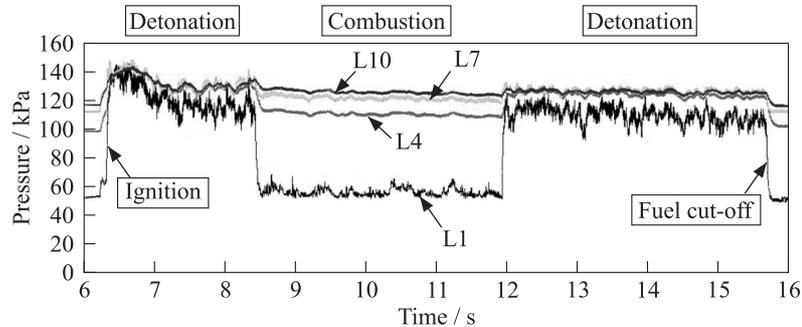
**Figure 2** Static pressure records in the CDA during one of the test fires with CSD–CPC–CSD mode transition
