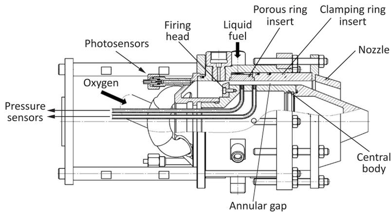
**Figure 1** Schematic of DLRE
