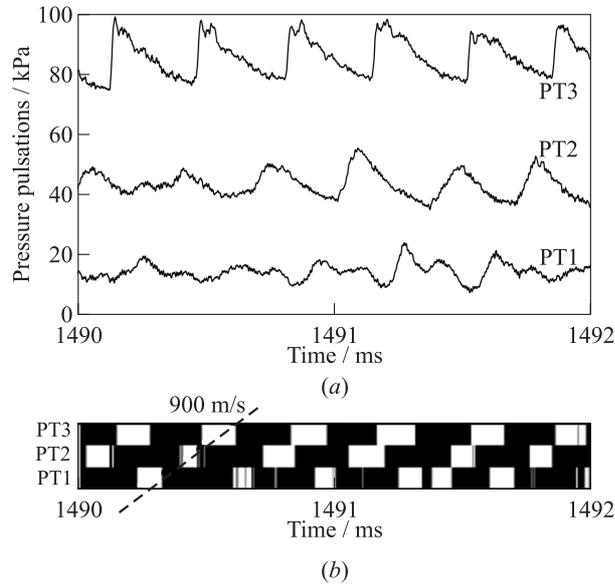
**Figure 8** A fragment of the records of high-frequency pressure sensors (a) and its visualization (b) for the CSD mode with a single rotating detonation wave
