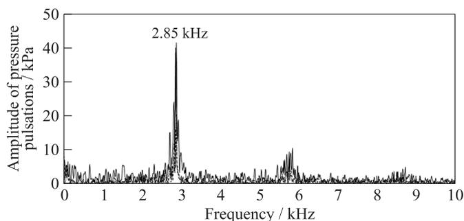
**Figure 6** Fourier transform of a fragment of records of three high-frequency pressure sensors
