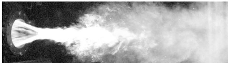
**Figure 4** Photo of the DLRE exhaust plume in one of the fire tests
