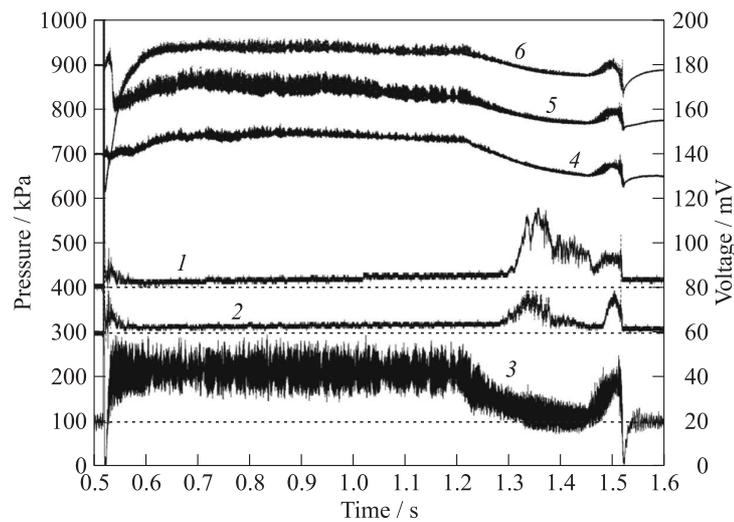
**Figure 5** Recordings of photosensors (1 and 2), static pressure sensor in the combustor (3), and high-frequency pressure sensors (4, 5, and 6) in one of the fire tests
