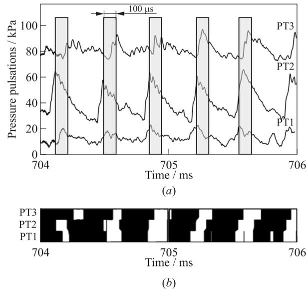
**Figure 7** A fragment of the records of high-frequency pressure sensors (a) and its “visualization” according to [27] (b) for the LPD mode
