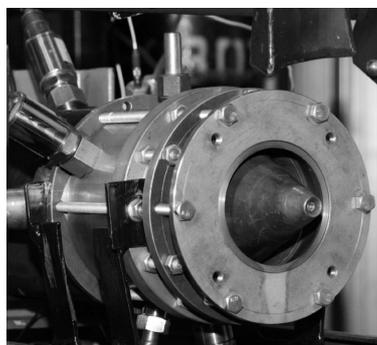
**Figure 2** Detonation LRE with the short nozzle attached
