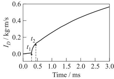
**Figure 3** The calculated temporal dependence of the total momentum of the detonation products at the inlet to the turbine
