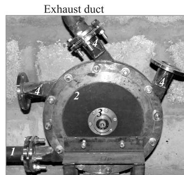
**Figure 8** Photograph of a pulse turbine connected to a pulse detonation tube and exhaust duct: 1 — pulse detonation tube; 2 — turbine housing; 3 — turbine shaft; and 4 — exhaust ports
