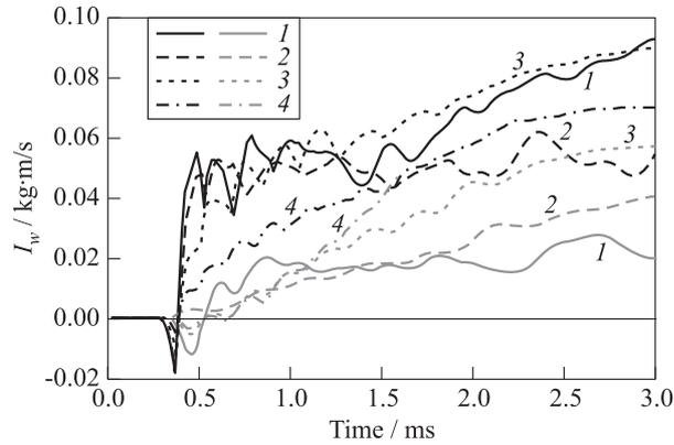
**Figure 5** Comparison of the calculated temporal dependencies of the momentum transferred to the rotor from the detonation products (black curves) and from the products of combustion at  $V = \text{const}$  (grey curves) for different values of the blockage factor  $\delta = 0.8$  (1), 0.6 (2), 0.4 (3), and 0.2 (4)
