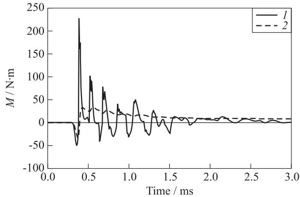
**Figure 6** An example of calculation of the instantaneous (1) and time-averaged (2) torque acting on the rotor of a pulse turbine in one operation cycle of a pulse detonation tube ( $\delta = 0.4$ )
