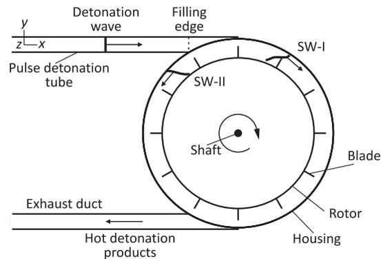
**Figure 1** Schematic of a pulse turbine for converting the kinetic energy of detonation products into rotational energy of a turbine rotor
