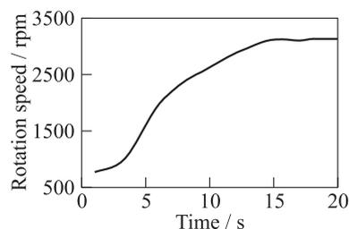
**Figure 9** Temporal dependence of the rotation speed of a pulse-turbine rotor at a detonation pulse frequency of 10 Hz
