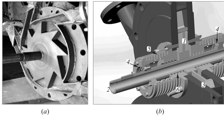
**Figure 7** Experimental sample of a pulse turbine: (a) photograph, (b) mount of the rotor; 1 — rotor with blades; 2 — shaft; 3 — housing; 4 — bearings; 5 — holders with cooling fins; and 6 — seals
