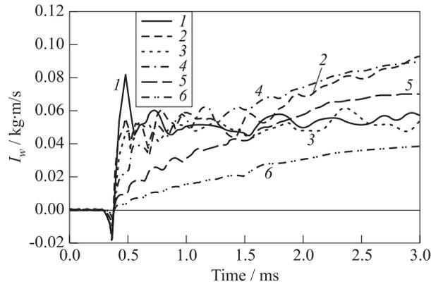
**Figure 4** The calculated temporal dependencies of the momentum transferred to the rotor from the detonation products for different values of the blockage factor: 1 —  $\delta = 0.9$ ; 2 — 0.8; 3 — 0.6; 4 — 0.4; 5 — 0.2, and 6 — 0.1
