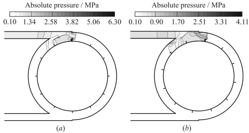
**Figure 2** Examples of calculated instantaneous pressure fields in the annular gap of a pulse turbine at the time when the SW entering the turbine reached the first rotor blade in the case of a stationary (a) and moving (b) rotor (rotation speed 4000 rpm) with a blockage ratio  $\delta = 0.2$
