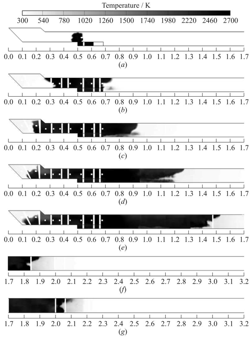
**Figure 5** The calculated gas temperature field in the middle longitudinal section of the inner path of the TM path at different time instants after prechamber ignition (check valve is closed): (a) 3 ms; (b) 5; (c) 6; (d) 7; (e) 7.5; (f) 8; and (g) 8.25 ms (*to be continued*)
