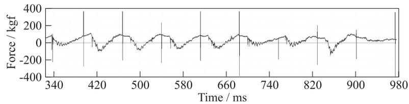
**Figure 9** An example of a primary record of a load cell in 10 successive cycles of a fire test at an operation frequency of 14 Hz
