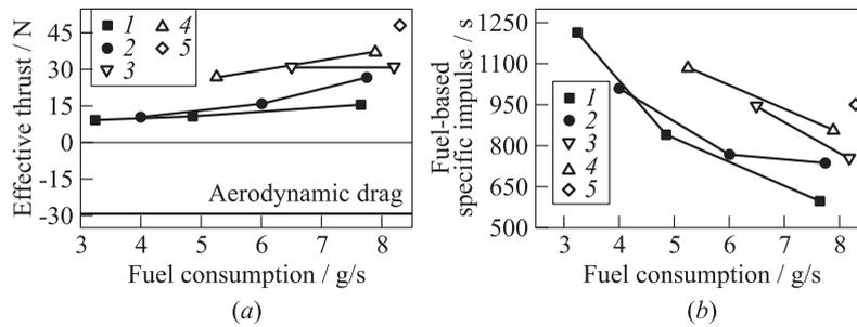
**Figure 10** Examples of measured thrust characteristics of the TM in terms of the dependencies of effective thrust and aerodynamic drag (a) and fuel-based specific impulse (b) on fuel consumption at the speed of the approaching air flow  $V = 65$  m/s: 1 —  $f = 4$  Hz; 2 — 5; 3 — 6.7; 4 — 10; and 5 —  $f = 14$  Hz
