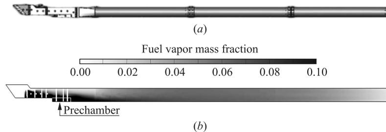
**Figure 4** The 3D model of TM (a) and an example of the calculated field of fuel vapor mass fraction in the inner path of the TM at the end of the filling stage of the detonation tube with a combustible mixture (check valve is open) (b)
