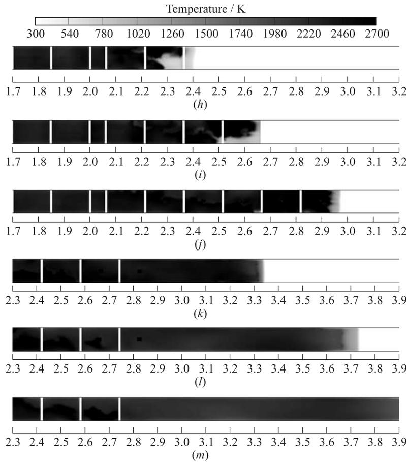
**Figure 5** (*continued*) The calculated gas temperature field in the middle longitudinal section of the inner path of the TM path at different time instants after prechamber ignition (check valve is closed): (h) 8.5 ms; (i) 8.75; (j) 9; (k) 9.25; (l) 9.5; and (m) 9.75 ms
