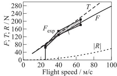
**Figure 12** Comparison of measured (shaded area) and calculated effective thrust  $F$  (solid curve) vs. flight speed for the 3-meter long TM with the detonation tube 110 mm in diameter. Dashed and dotted curves show the calculated full thrust  $T$  and aerodynamic drag  $R$  forces
