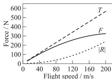
**Figure 3** Calculated thrust parameters vs. flight speed for the 3-meter long TM with  $100 \times 100$  mm cross-sectional area
