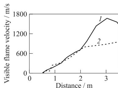
**Figure 6** Comparison of calculated dependencies of the apparent flame front velocity on the traversed (axial) distance for two variants of the TM: 1 — with DDT; and 2 — without DDT
