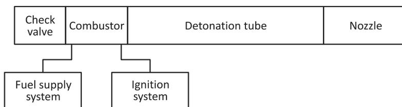
**Figure 1** Schematic diagram of the TM
