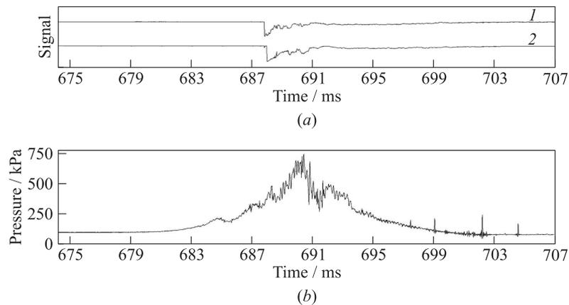
**Figure 8** Example of primary records of ionization probes (curves 1 and 2) (a) and a low-frequency pressure sensor at the check valve (b) in a fire test of TM with an operation frequency of 4 Hz
