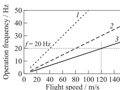
**Figure 2** Calculated dependencies of the operation frequency on the flight speed for the TM of different lengths: 1 —  $L = 1$  m; 2 —
