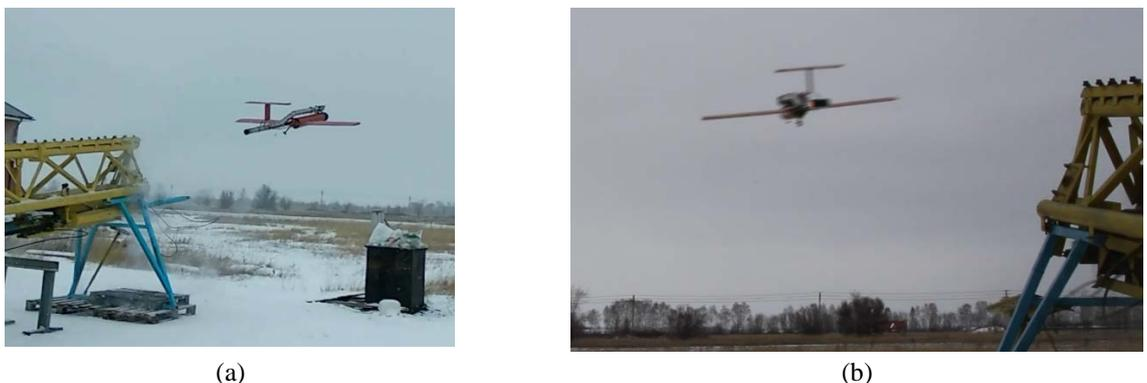
Figure 2: The UAVs powered with one TM (a) and two paired TMs (b) in the flight
