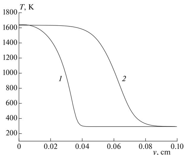
**Fig. 6.** Calculated temperature profiles in the (1) laminar and (2) turbulent flames. Hydrogen–air mixture, fuel–air equivalence ratio  $\Phi = 0.5$ , initial temperature  $T_0 = 293$  K, and atmospheric pressure. The turbulence characteristics for the turbulent flame are  $\bar{u} = 1100$  cm/s,  $L' = 1$  cm,  $L'' = 0.7$  cm, and  $\tau = 0.010$  s.
