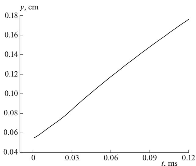
**Fig. 4.** Calculated dependence of the distance travelled by the averaged turbulent flame front on time. Hydrogen–air mixture; fuel–air equivalence ratio  $\Phi = 0.5$ ; initial temperature  $T_0 = 293$  K; atmospheric pressure; and turbulence characteristics:  $\bar{u} = 660$  cm/s,  $L' = 1$  cm,  $L'' = 0.7$  cm, and  $\tau = 0.010$  s.
