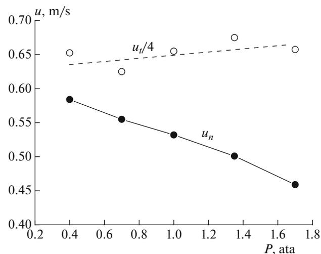
**Fig. 9.** Calculated dependences of the laminar flame propagation velocity  $u_n$  and the turbulent flame propagation velocity  $u_t$  on pressure. Hydrogen–air mixture, fuel–air equivalence ratio  $\Phi = 0.5$ , and initial temperature  $T_0 = 293$  K. Turbulence characteristics for  $u_i$ :  $\bar{u} = 510$  cm/s,  $L = 1$  cm,  $L' = 0.7$  cm, and  $\tau = 0.010$  s.
