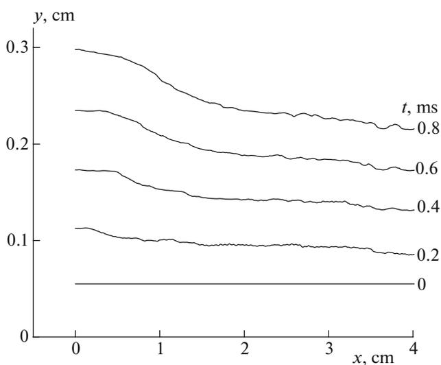
**Fig. 3.** Calculated positions of the turbulent flame front in various times ( $t = 0$ – $0.8$  ms). Hydrogen–air mixture; fuel–air equivalence ratio  $\Phi = 0.5$  ( $H_2$  volume content 17.36%); initial temperature  $T_0 = 293$  K; atmospheric pressure; and turbulence characteristics:  $\bar{u} = 130$  cm/s,  $L' = 1$  cm,  $L'' = 0.7$  cm, and  $\tau = 0.010$  s.
