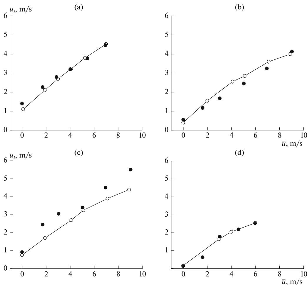
**Fig. 5.** Calculated (filled circles) and measured [18] (open circles with lines) dependences of the turbulent flame propagation velocity  $u_t$  on the root-mean-square pulsation velocity  $\bar{u}$ . Hydrogen-air mixtures containing (a) 23.09, (b) 13.51, (c) 17.36, and (d) 9.09% H<sub>2</sub>; initial temperature  $T_0 = 293$  K; atmospheric pressure; and turbulence characteristics:  $L = 1$  cm,  $L' = 0.7$  cm, and  $\tau = 0.010$  s.
