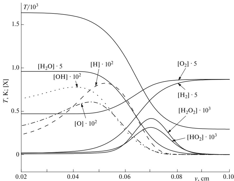
**Fig. 7.** Calculated profiles of temperature and the concentrations (volume fractions)  $[X]$  of some species in the turbulent flame. Hydrogen–air mixture; fuel–air equivalence ratio  $\Phi = 0.5$ ; initial temperature  $T_0 = 293$  K; atmospheric pressure; and turbulence characteristics:  $\bar{u} = 1100$  cm/s,  $L' = 1$  cm,  $L'' = 0.7$  cm, and  $\tau = 0.010$  s.
