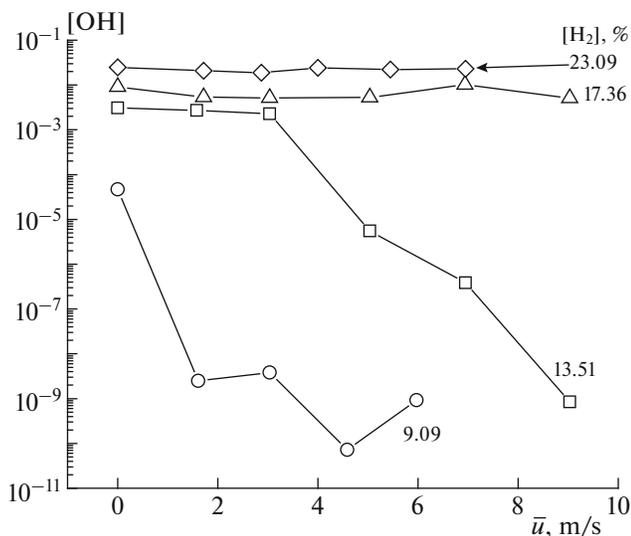
**Fig. 8.** Calculated dependences of the hydroxyl concentration (volume fraction)  $[\text{OH}]$  on the root-mean-square pulsation velocity  $\bar{u}$ . Hydrogen–air mixtures of various compositions; initial temperature  $T_0 = 293$  K; atmospheric pressure; and turbulence characteristics:  $L = 1$  cm,  $L' = 0.7$  cm, and  $\tau = 0.010$  s.
