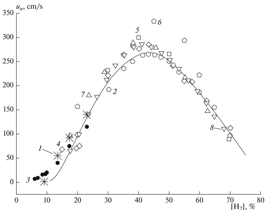
**Fig. 2.** Comparison of the calculated and measured values of the laminar flame propagation velocity  $u_n$  on the composition of the hydrogen–air mixture. Initial temperature  $T_0 = 293$  K, atmospheric pressure. (1) Results of calculations in this work and experimental points (2) [3], (3) [18], (4) [19], (5) [20], (6) [21], (7) [22], and (8) [23]; the curve represents the results of the calculation [24].
