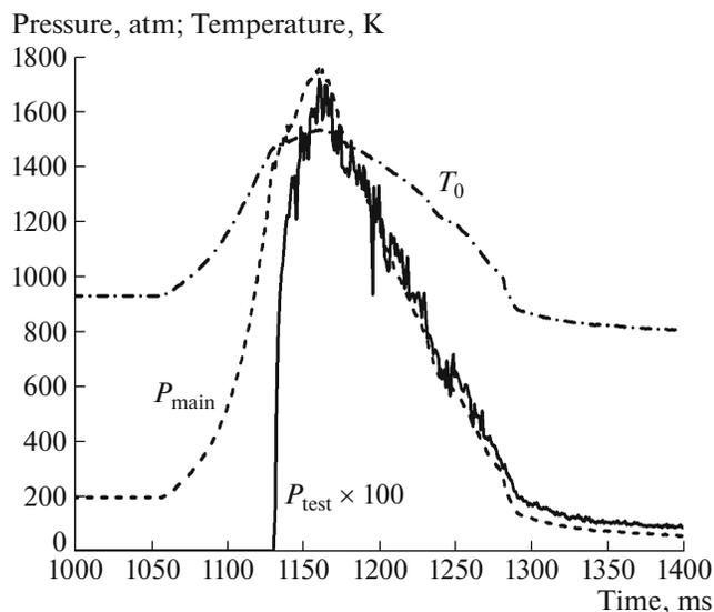
**Fig. 2.** Time dependence of the air pressures  $P_{\text{main}}$  and  $P_{\text{test}}$  in the main and test prechambers of the wind tunnel, respectively, and the air temperature  $T_0$  in these prechambers.
