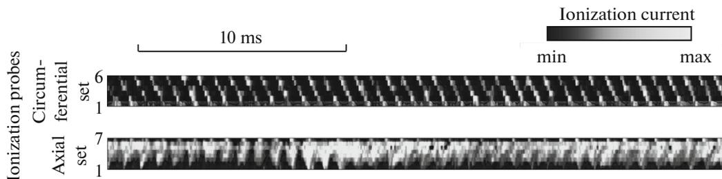
**Fig. 3.** Example of the visualization of the readings of the ionization probes in the fire test of the DABR model in a continuous spinning detonation mode.
