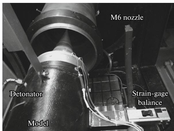
**Fig. 1.** Photograph of the DABR model in the test section of the AT-303 impulse wind tunnel.
