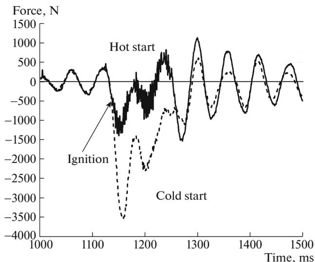
Fig. 4. Example of the records of the instantaneous forces acting on the DABR model during the cold (dashed curve) and hot (solid curve) starts.
