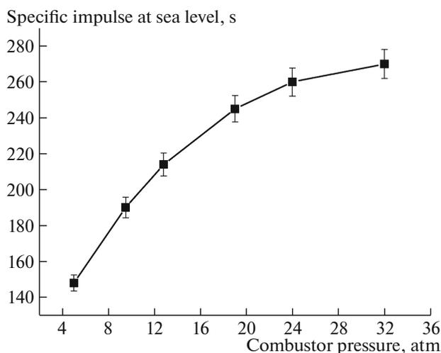
Fig. 4. Experimental dependence of the specific impulse at sea level on the mean static pressure in the DRE combustor.
