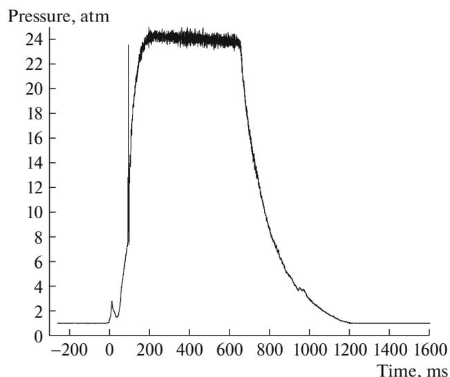
**Fig. 2.** Example of the readings of the static pressure sensor in the DRE combustor.
