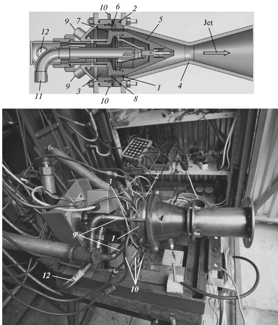
Fig. 1. Schematic of the DRE and a photograph of its installation on a test stand.
