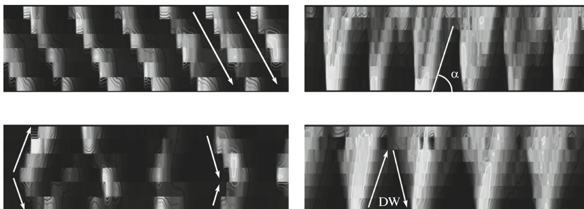
**Fig. 2.** Visualization of the readings of the ionization probes in the form of the circumferential (left) and longitudinal (right) unfolded views in the modes of CSD (top) and LPD (bottom) of hydrogen in the combustor of the ABR demonstrator. DW stands for detonation wave.
