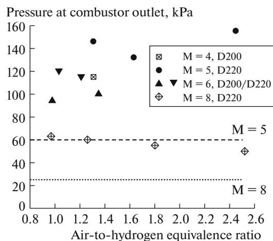
**Fig. 4.** Dependence of the total pressure at the combustor outlet on air-to-hydrogen equivalence ratio in the fire tests of the ABR demonstrator with throttle discs D200 and D220 (points at Mach 4, 5, 6, and 8) and in the cold blowing with throttle disc D220 (dashed and dotted horizontal lines at Mach 5 and 8, respectively).
