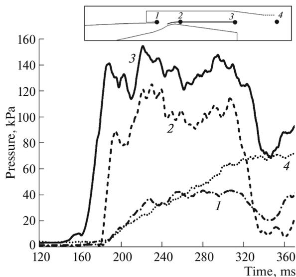
**Fig. 3.** Readings of (1) the total pressure at the nozzle outlet section, (2) the static pressure at the combustor inlet, (3) the total pressure at the combustor outlet, and (4) the static pressure in the vacuum chamber of the wind tunnel. Points 1–4 indicate the positions of the respective sensors.
