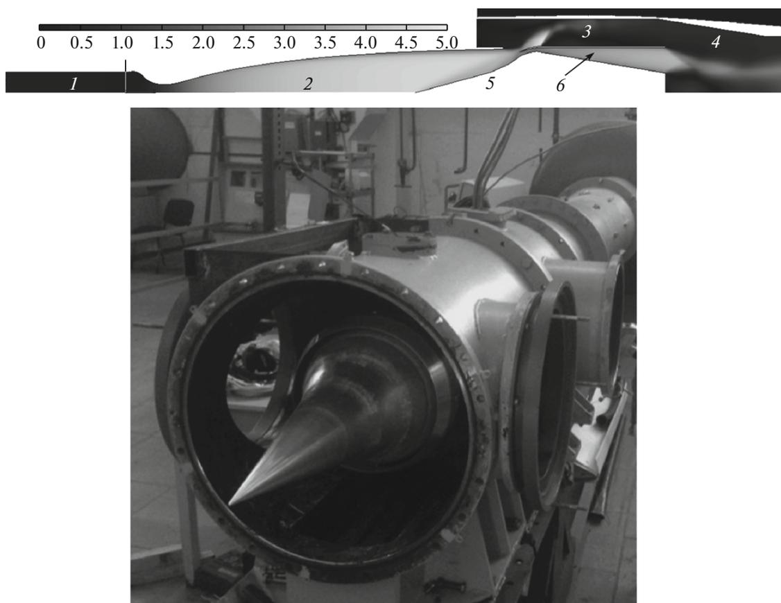
**Fig. 1.** Photograph of the flow duct of the wind tunnel with the mounted ABR demonstrator and the calculated local Mach number distribution while blowing with an air flow at Mach 5. The numbers indicate the main parts of the setup: (1) prechamber, (2) axisymmetric supersonic nozzle, (3) test section of the wind tunnel, (4) diffuser, (5) air intake, and (6) combustor of the ABR demonstrator.
