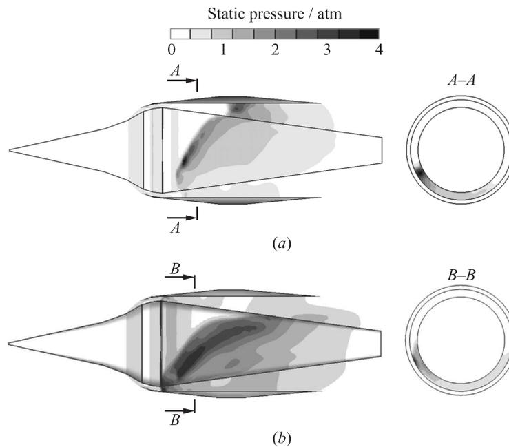
**Figure 3** Calculated fields of static pressure on the surface of the central body and in the annular channel of the combustor for variants 3 (a) and 5 (b). In sections A-A and B-B, the detonation wave rotates clockwise
