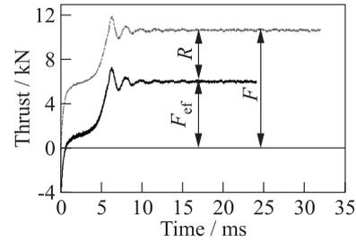
**Figure 2** Approach of the engine thrust  $F$  and the efficient thrust of the power plant to their steady-state values for variant 5
