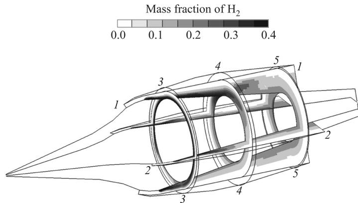
**Figure 4** Calculated fields of hydrogen mass fraction in various longitudinal (1-1 and 2-2) and transverse (3-3, 4-4, and 5-5) sections for variant 5
