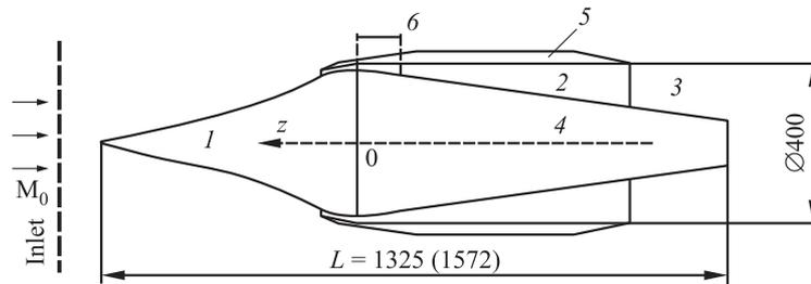
**Figure 1** Schematic diagram of a ramjet power plant with a continuous-detonation combustor (for details, see the text). Dimensions are in millimeters
