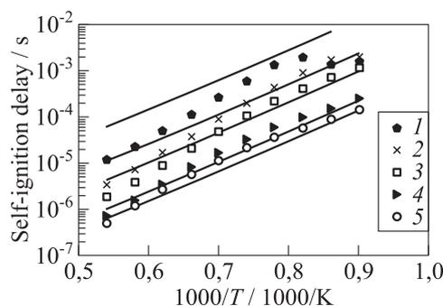
**Figure 2** Example of calculated dependences of self-ignition delay on the initial temperature at different initial pressures obtained by mechanism (I)–(V) (curves) and DKM (symbols) at  $\Phi = 1$ : 1 —  $P = 1$  atm; 2 — 5; 3 — 12; 4 — 50; and 5 —  $P = 80$  atm
