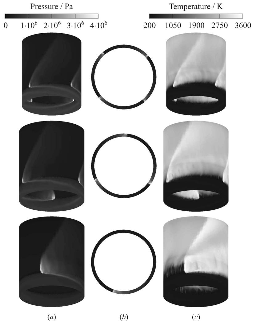
**Figure 3** Predicted quasi-stationary fields of static pressure (*a* and *b*) and static temperature (*c*) under the conditions of experimental Tests 2 (upper row), 3 (middle row), and 4 (bottom row)
