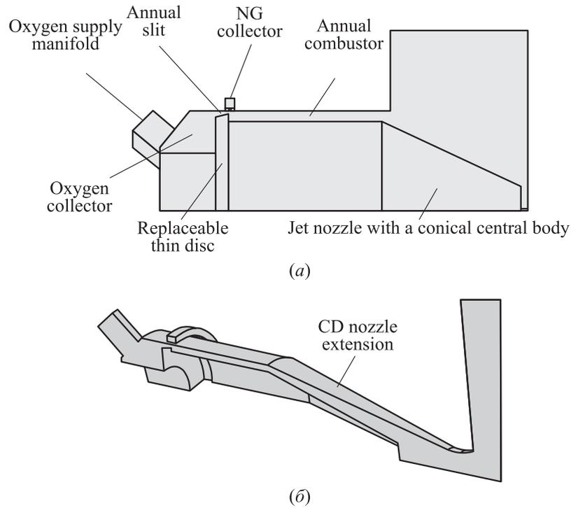
**Figure 1** Longitudinal section (a) and a perspective view of a quarter (b) of DLRE of two different configurations with oxygen and NG collectors and pieces of oxygen-feeding manifold
