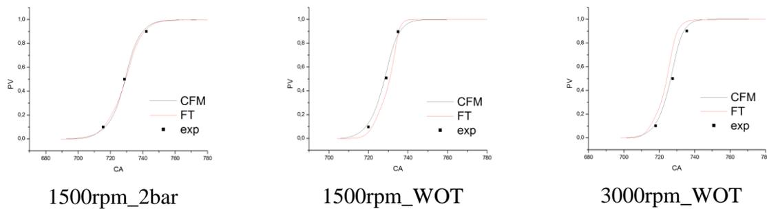
Figure 1: Comparative performances of the new ignition/combustion model (black curves) and standard CFM model (red curves) in terms of the Progress Variable vs. Crank Angle dependences against experimental points for a particular IC engine at different loading conditions.
