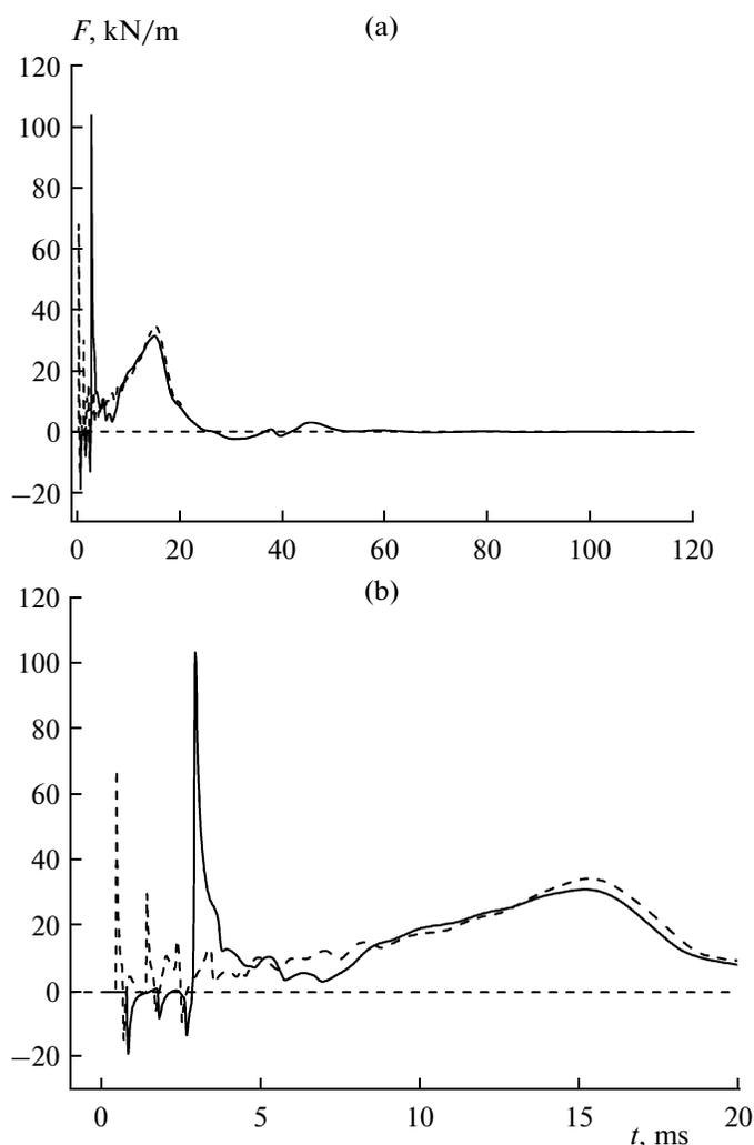
**Fig. 8.** Calculated time evolution of the instantaneous force acting on the device during momentum transfer from a shock wave to a bubbly water charge with  $\alpha_{20} = 0.9$  (solid line) and to a continuous water charge with  $\alpha_{20} = 1$  (dashed line): (a) flow duration is 120 ms, (b) initial 20-ms portion of (a).
