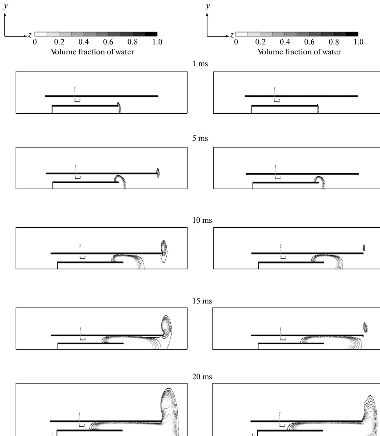
**Fig. 7.** Calculated isolines of the volume fraction of water  $\alpha_2$  at different points in time after the opening of the diaphragm in the shock wave generator (plotted at a step of 0.1). Panels on the left refer to a bubbly water charge with  $\alpha_{20} = 0.9$ ; those on the right, to a continuous water charge,  $\alpha_{20} = 1$ .
