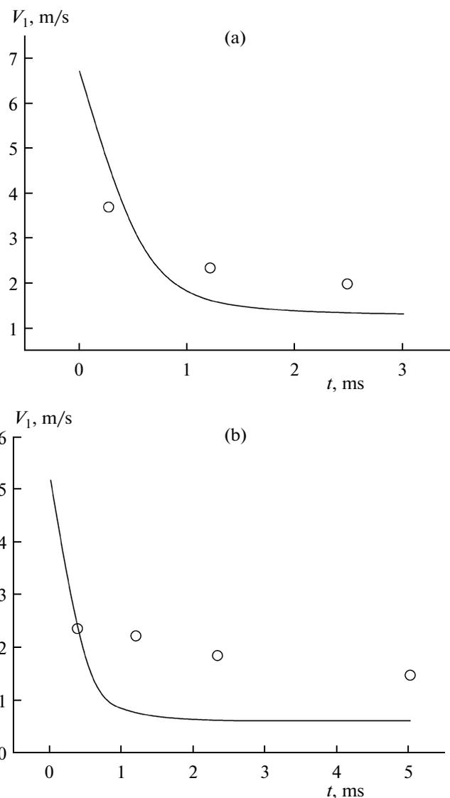
Fig. 5. Comparison of the calculation results (curves, present work) with the experimental data (symbols) [16] on the time evolution of the velocity of a gas bubble set in motion by a shock wave: (a) run 1, (b) run 2 in Table 2.
