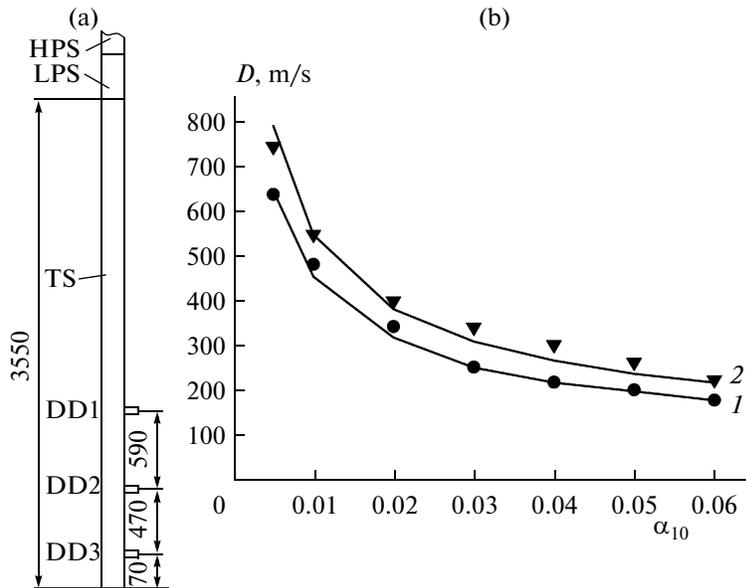
Fig. 3. (a) Schematic of the experimental setup used in [14] (dimensions in mm); (b) comparison of the calculated (curves, present work) and measured (symbols [14]) dependences of the shock-wave velocity within measurement segments DD1–DD2 and DD2–DD3 on the volume fraction  $\alpha_{10}$  of air bubbles in the water at different pressures in the HPS: (●, 1)  $p_{HPS} = 24$  atm and (▼, 2) 36 atm.
