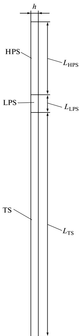
Fig. 1. Schematic diagram of the shock tubes used in [13–16] to study the propagation of shock waves in bubbly liquids.
