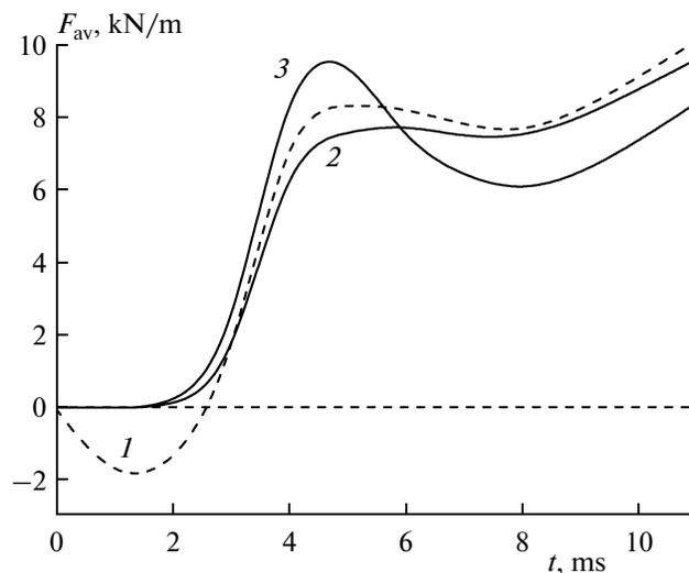
**Fig. 10.** Calculated time histories of the average force acting on the device for three variants of filling of the water duct with bubbly liquid with  $\alpha_{20} = 0.9$ : (1) only region I (Fig. 6) is filled; (2) regions I and II, and (3) regions I, II, and III.
