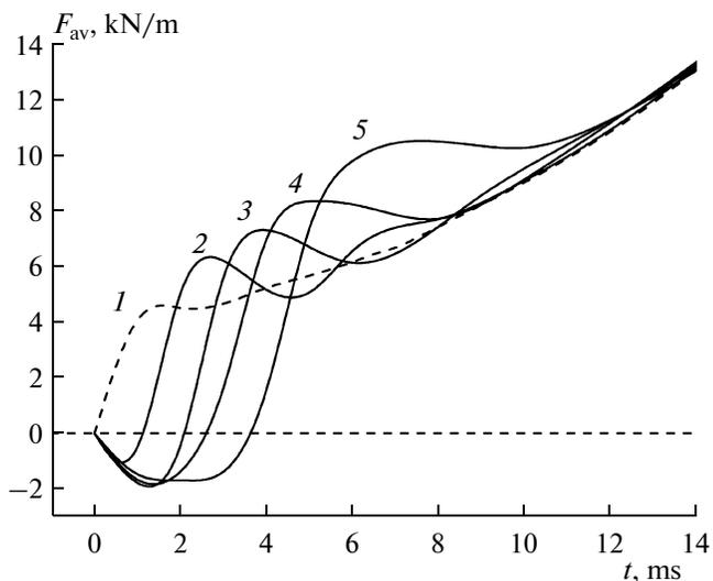
**Fig. 9.** Calculated time histories of the average force exerted on the device during momentum transfer from a shock wave to (1) a continuous water charge ( $\alpha_{20} = 1$ ) and to bubbly water charges with  $\alpha_{20} =$  (2) 0.97, (3) 0.94, (4) 0.9, and (5) 0.8.
