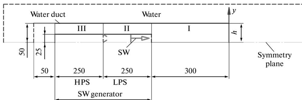
**Fig. 6.** Schematic diagram of the model device for calculating the momentum transfer from a shock wave to a bubbly medium (dimensions in mm).
