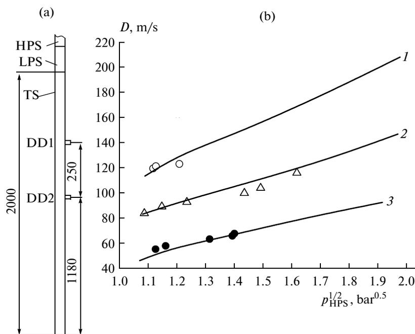
**Fig. 4.** (a) Schematic diagram of the experimental setup used in [15] (dimensions in mm); (b) comparison of the calculated (curves, present work) and measured (symbols [15]) dependences of the shock-wave velocity within measurement segment DD1–DD2 on the pressure in the HPS  $p_{\text{HPS}}$  at different initial volume fraction of air bubbles  $\alpha_{10}$  in water–glycerol solutions: ( $\circ$ , 1) 0.01, ( $\triangle$ , 2) 0.02, and ( $\bullet$ , 3) 0.05.
