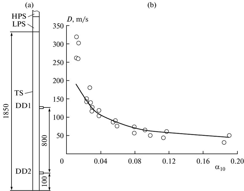
Fig. 2. (a) Schematic diagram of the experimental setup used in [13] (dimensions in mm); (b) comparison of the calculated (curve, present work) and measured (symbols [13]) dependences of the shock wave velocity within measurement segment DD1–DD2 on the volume fraction of air bubbles in the water.
