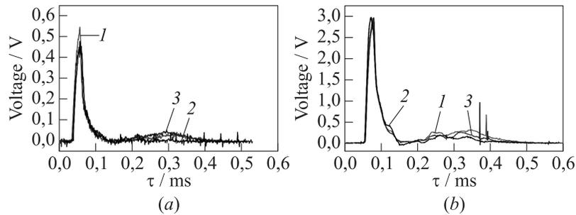
**Figure 4** Typical records of voltage pulse at electrodes 1 as a function of operation frequency (1 — 20 Hz; 2 — 30; and 3 — 40 Hz); magnetic induction 0.6 T; load 1 Ohm (a) and 10 Ohm (b)
