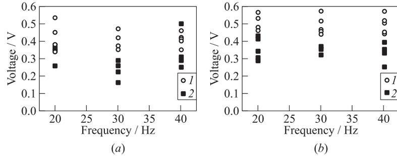
**Figure 3** Effect of operation frequency on the measured voltage magnitude at MHD-channel electrodes (1 — electrode 1 and 2 — electrode 2); magnetic induction 0.6 T; load 1 Ohm (a) and 10 Ohm (b)
