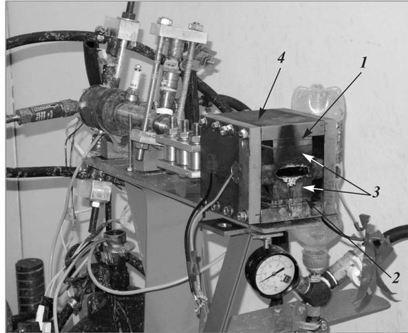
**Figure 5** Photo of the MHD-channel with aluminum inserts: 1 — upper insert; 2 — lower insert; 3 — permanent magnets; and 4 — magnetic circuit
