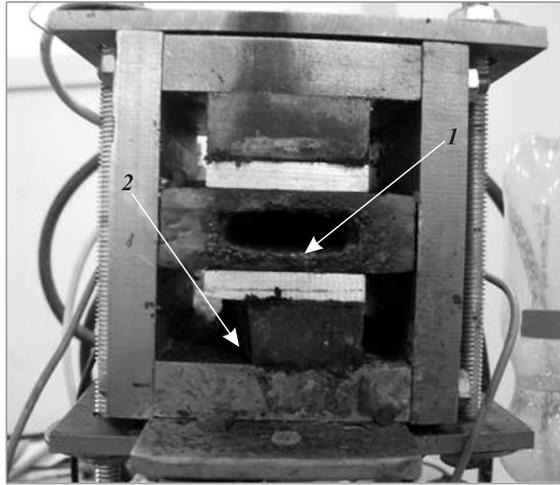
**Figure 2** Photo of the MHD-channel exit section at the end of experimental campaign (*1* — mechanical damage of the inner wall; and *2* — mechanical damage of the magnet)
