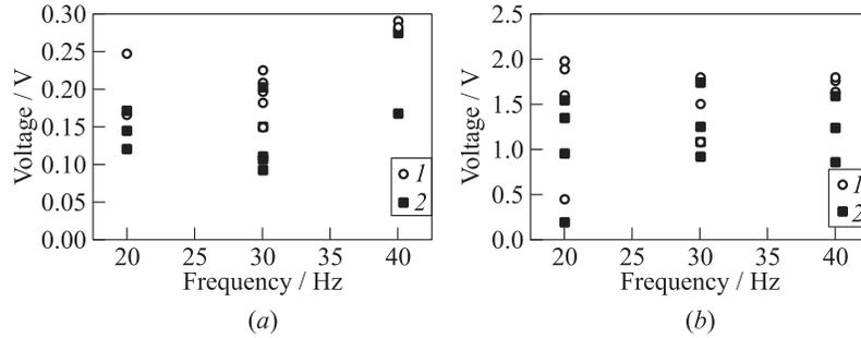
**Figure 6** Effect of operation frequency on the voltage magnitude at MHD-channel electrodes (1 — electrode 1 and 2 — electrode 2); magnetic induction 0.3 T; load 1 Ohm (a) and 10 Ohm (b)
