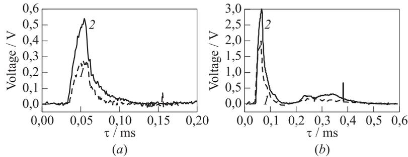
**Figure 7** Typical records of voltage pulse at electrodes 1 as a function of magnetic induction (1 — 0.3 T and 2 — 0.6 T) at operation frequency 20 Hz; load 1 Ohm (a) and 10 Ohm (b)
