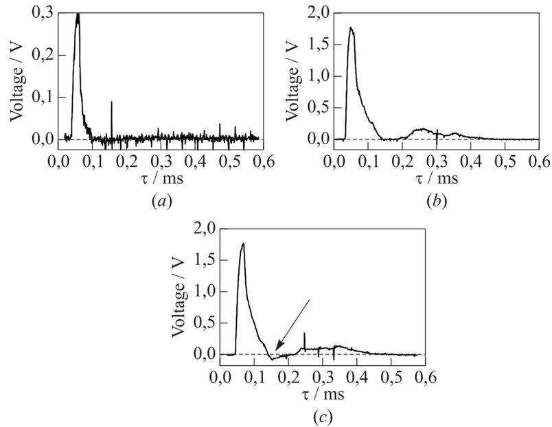
**Figure 8** Three types of MHD voltage signals: (a) single-peak; (b) double-peak; and (c) double-peak with sign reversal
