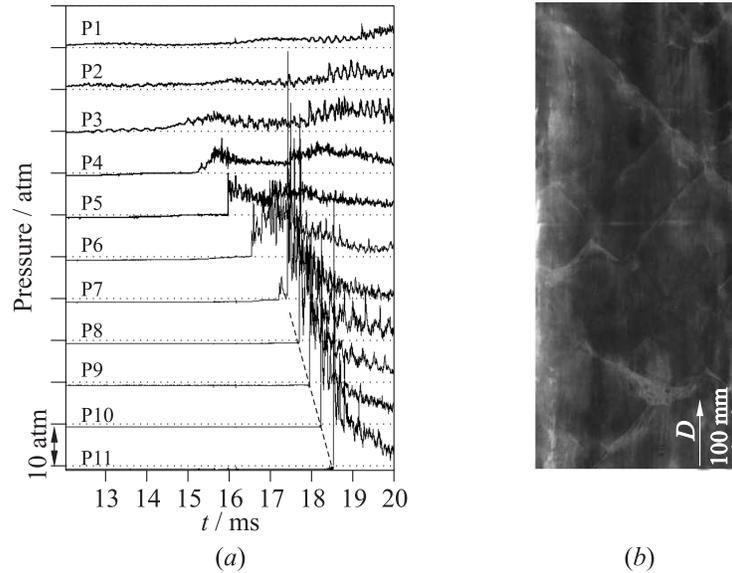
**Figure 2** Pressure records by sensors P1 to P11 in one of PDC operation cycles in an experiment with fast cyclic DDT at  $(1.8 \pm 0.1)$  Hz (dashed line shows the detonation wave trajectory) (a) and the photograph of the smoked foil footprint of the detonation in a single shot (b)
