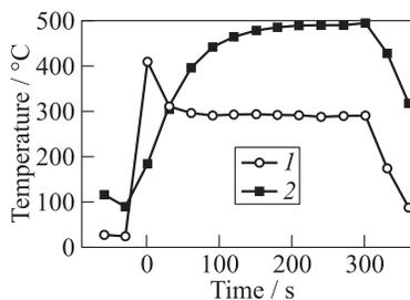
**Figure 4** The measured temperature histories of different structural elements of the PDB in the experiment with the operation frequency of  $(1.8 \pm 0.1)$  Hz and with the duration of 300 s: 1 — interior obstacle in the burner duct (position 3 in Fig. 1); and 2 — interior obstacle (position 5)
