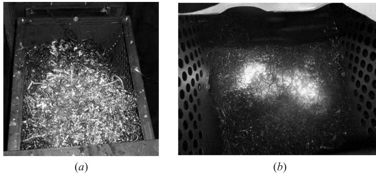
**Figure 6** Metal shavings before (a) and after (b) the 100-second impact of PDB jets
