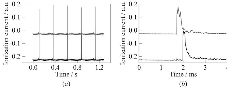
**Figure 3** Records of two ionization probes located at a distance of 0.5 m from each other in the part of PDB duct with periodic passage of detonations: (a) original records; and (b) resolution of the peaks of ionization current in the millisecond range
