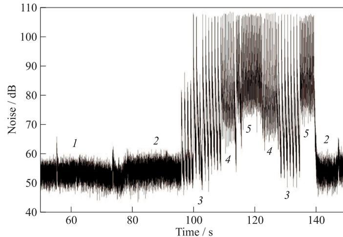
**Figure 5** The PDB noise level at the outlet of furnace chimney
