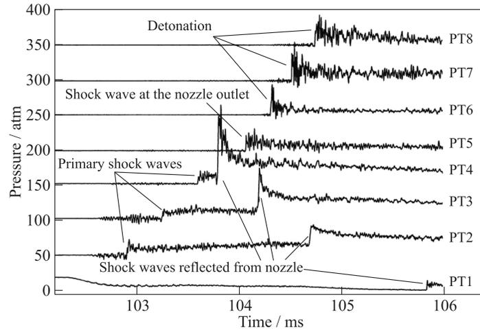
**Figure 3** Pressure records of transducers PT1–PT8 in one of representative experiments (curve 1 in Fig. 2) with identification of wave phenomena
