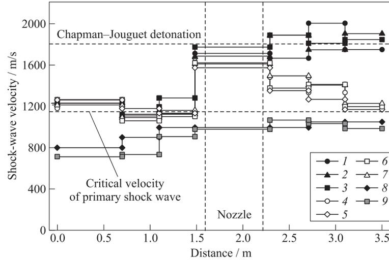
**Figure 2** Average velocity of the lead shock front vs. travelled distance in various measuring segments in 9 representative experiments. Distance is measured from PT1
