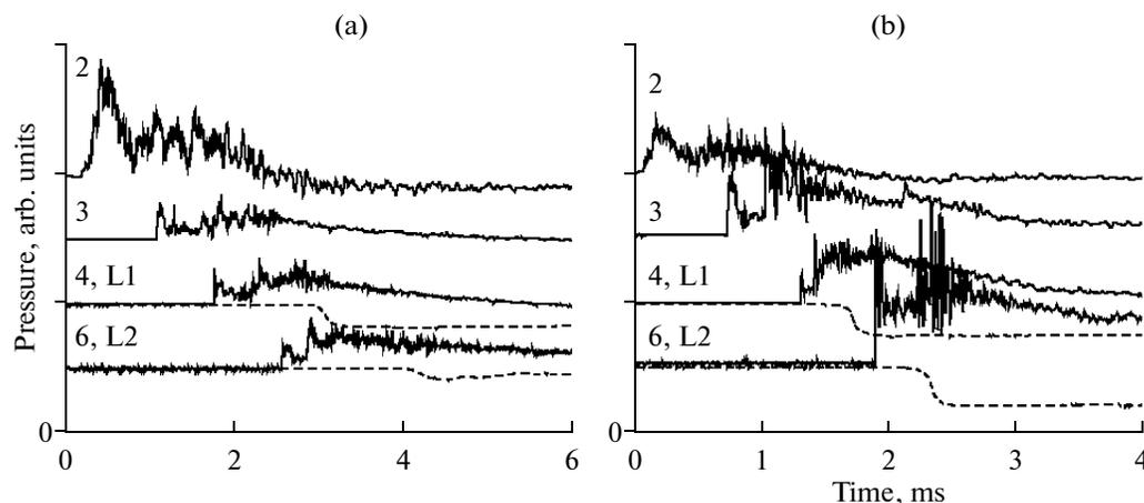
**Fig. 2.** Pressure profiles recorded by sensors 2–4 and 6 (solid curves) and luminescence intensity profiles recorded by photodiodes L1 and L2 (dashed curves) in experiments (a) I and (b) II.
