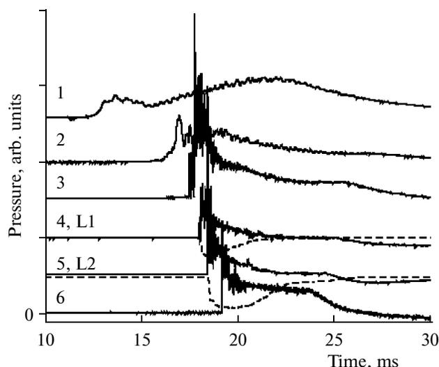
**Fig. 4.** Pressure profiles recorded by sensors 1–6 (solid curves) and luminescence intensity profiles recorded by photodiodes L1 and L2 (dashed curves) in experiment V.
