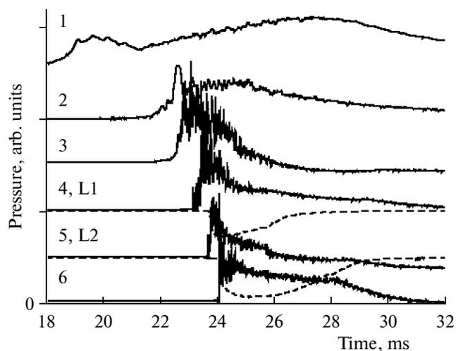
**Fig. 5.** Pressure profiles recorded by sensors 1–6 (solid curves) and luminescence intensity profiles recorded by photodiodes L1 and L2 (dashed curves) in experiment VI.
