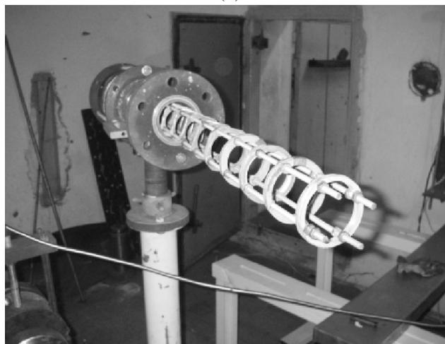
Fig. 1. (a) Schematic diagram of the experimental setup and (b) photograph of turbulizing obstacles.
