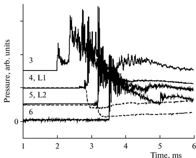
Fig. 3. Pressure profiles recorded by sensors 3–6 (solid curves) and luminescence intensity profiles recorded by photodiodes L1 and L2 (dashed curves) in experiment IV.
