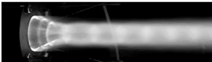
**Figure 2** Photo of supersonic jet issuing from the LRE prototype nozzle
