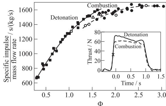
**Figure 4** The ratio of specific impulse to fuel–mixture mass flow rate vs. mixture composition. Insert shows time histories of thrust at engine operation in the continuous-detonation mode (0.056 kg/s,  $\Phi = 1.55$ ) and continuous-combustion mode (0.053 kg/s,  $\Phi = 1.75$ )
