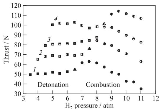
**Figure 3** Thrust vs. hydrogen supply pressure at different oxygen supply pressures: series 1 — 3.5 atm; 2 — 4; 3 — 4.5; and series 4 — 5 atm
