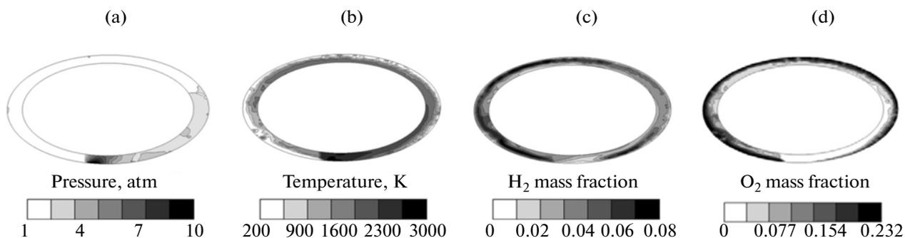
**Fig. 4.** Instantaneous distributions of (a) pressure, (b) temperature, and (c) hydrogen and (d) oxygen mass fractions at a cross section  $z = 40$  mm from the RDC bottom. Detonation propagates from the right to the left. Variant 1.
