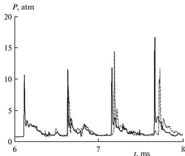
**Fig. 13.** Comparison of the calculated time dependences of the static pressure at a point located at the external wall of the RDC at a distance of  $z = 40$  mm for the coarse (solid curve) and fine (dashed) computational grid. Variant 1.
