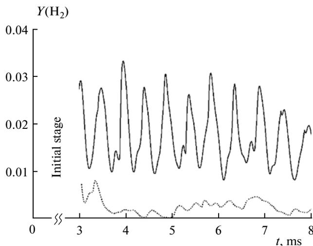
**Fig. 10.** Calculated time dependences of the hydrogen mass fraction at a point of middle cross section of the RDC at a distance of  $z = 350$  mm from the bottom for variants 1 (solid) and 2 (dashed curve).
