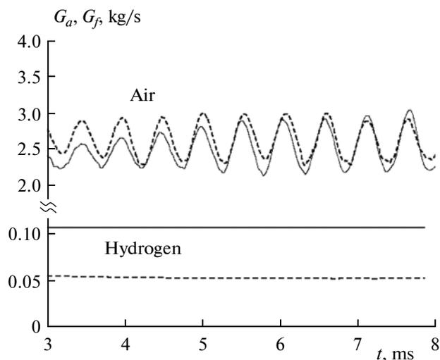
**Fig. 12.** Comparison of the calculated time dependences of the mass flow rates of air and hydrogen for variants 1 (solid curve) and 2 (dashed).
