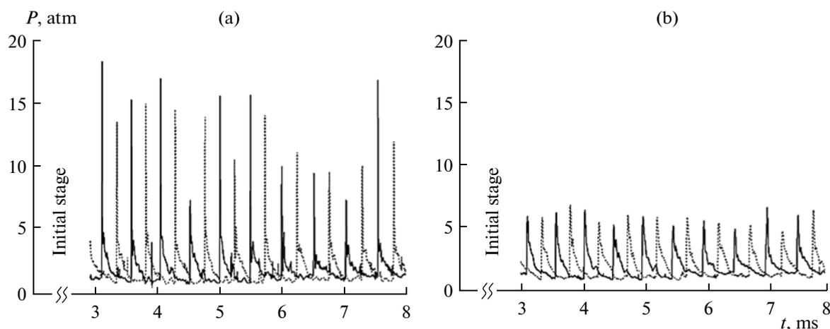
**Fig. 8.** Calculated time dependences of the static pressure at two points located in the RDC a distance of  $z = 40$  mm from the bottom  $180^\circ$  apart (solid and dashed curves) at the (a) external and (b) internal walls. Variant 1.
