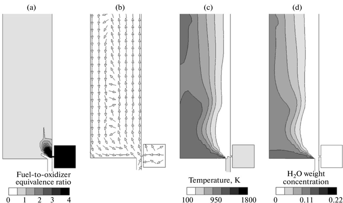
**Fig. 11.** Instantaneous distributions of (a) fuel-to-oxidizer equivalence ratio, (b) velocity, (c) temperature, and (d) water vapor mass fraction in the longitudinal section of the RDC at a time immediately before detonation wave arrival. Variant 2.
