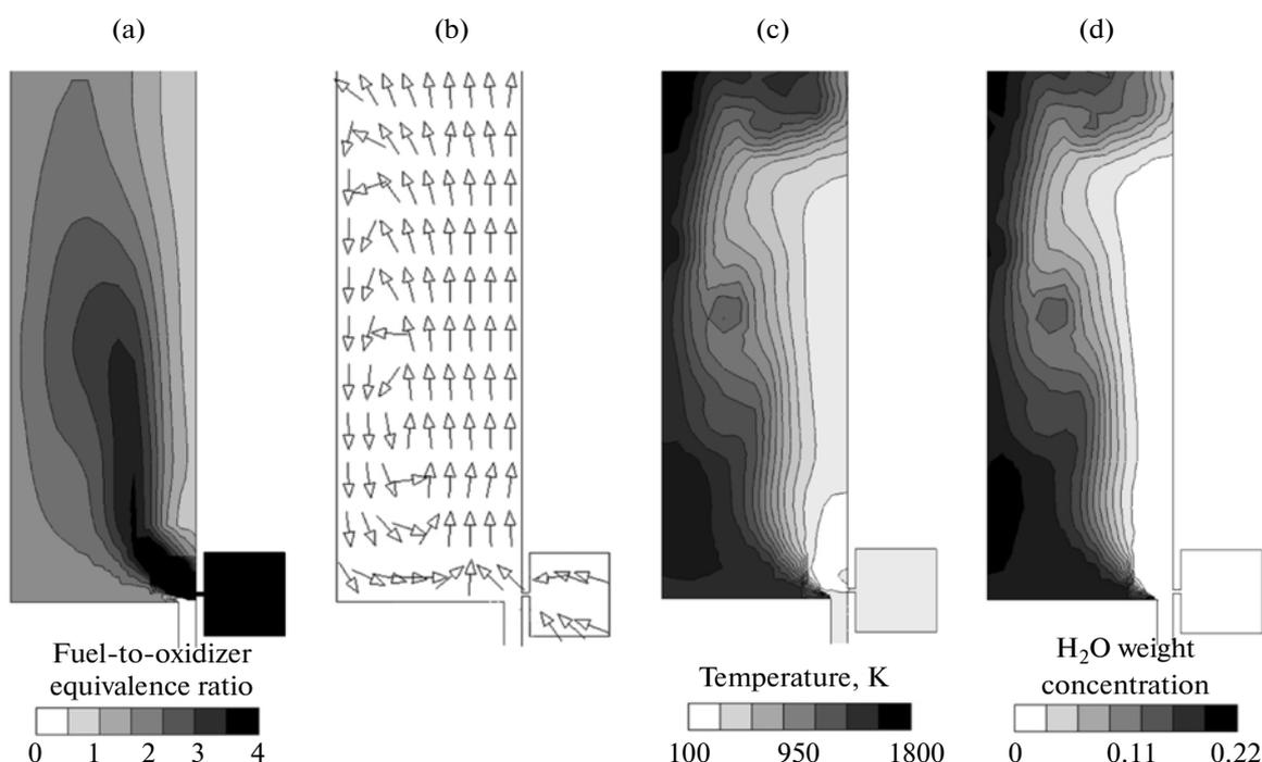
**Fig. 9.** Instantaneous distributions of (a) fuel-to-oxidizer equivalence ratio, (b) velocity, (c) temperature, and (d) water vapor mass fraction in the longitudinal section of the RDC at a time immediately before detonation wave arrival. Variant 1.
