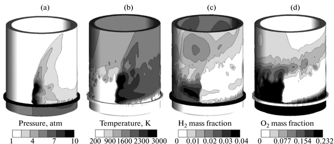
**Fig. 3.** Instantaneous distributions of (a) pressure, (b) temperature, and (c) hydrogen and (d) oxygen mass fractions, near the external wall of an RDC operating in the mode of separate supply of air and hydrogen. Detonation propagates from the right to the left. Variant 1.
