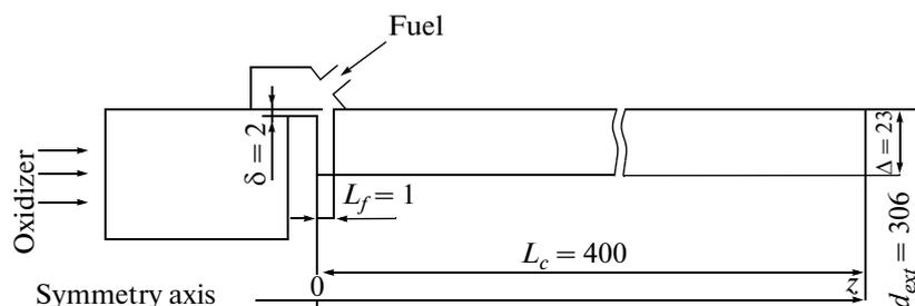
Fig. 1. Dimensions (in mm) of the rotating detonation chamber.
