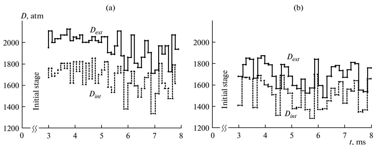
**Fig. 7.** Detonation velocity at the external (solid lines) and internal (dashed lines) walls of the RDC as a function of the time for variants (a) 1 and (b) 2 at a distance of  $z = 40$  mm from the chamber bottom.
