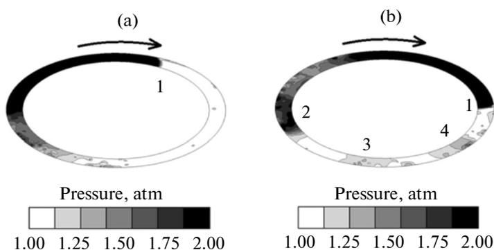
**Fig. 5.** Instantaneous distributions of (a) pressure, (b) temperature, and (c) hydrogen and (d) oxygen mass fractions at a cross section  $z = 40$  mm from the RDC bottom at times  $t =$  (a) 2.90 and (b) 6.86 ms, when only one detonation wave (1) propagates, without other supersonic reaction fronts (a) and when there are three additional reaction fronts (2, 3, 4) (b). Detonation propagates clockwise. Variant 1.
