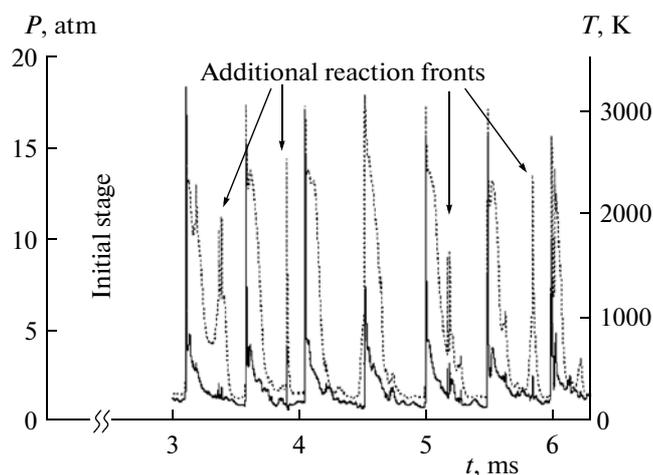
**Fig. 6.** Calculated time dependences of the static pressure (solid curve) and static temperature (dashed curve) at a point located at the external wall of the RDC at a distance of  $z = 40$  mm from the bottom. Variant 1.
