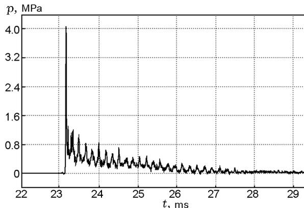
**Fig. 9.** Oscillogram of pressure in the spin detonation wave.
