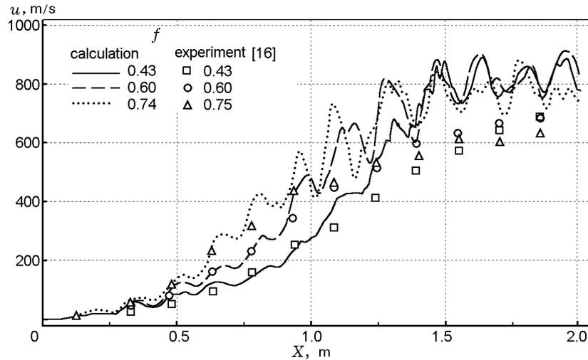
**Fig. 2.** Comparison of the calculated (curves) and experimental [16] (points) of the visible velocity of the flame front versus the covered distance.
