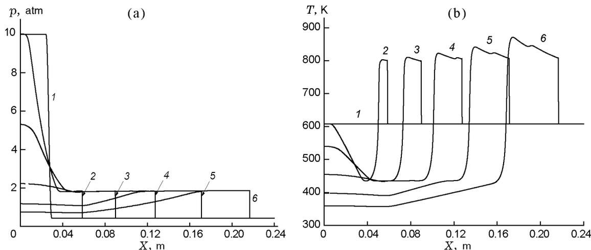
**Fig. 6.** Calculated profiles of pressure (a) and temperature (b) in the shock wave without preliminary thermal treatment of the mixture ( $C_5H_{12}:8O_2$ ):  $T_0 = 608$  K,  $p_0 = 0.42$  atm,  $t_i = 0$ , and  $t = 0$  (1), 43.4 (2), 87.2 (3), 141 (4), 204 (5), and 270  $\mu$ s (6).
