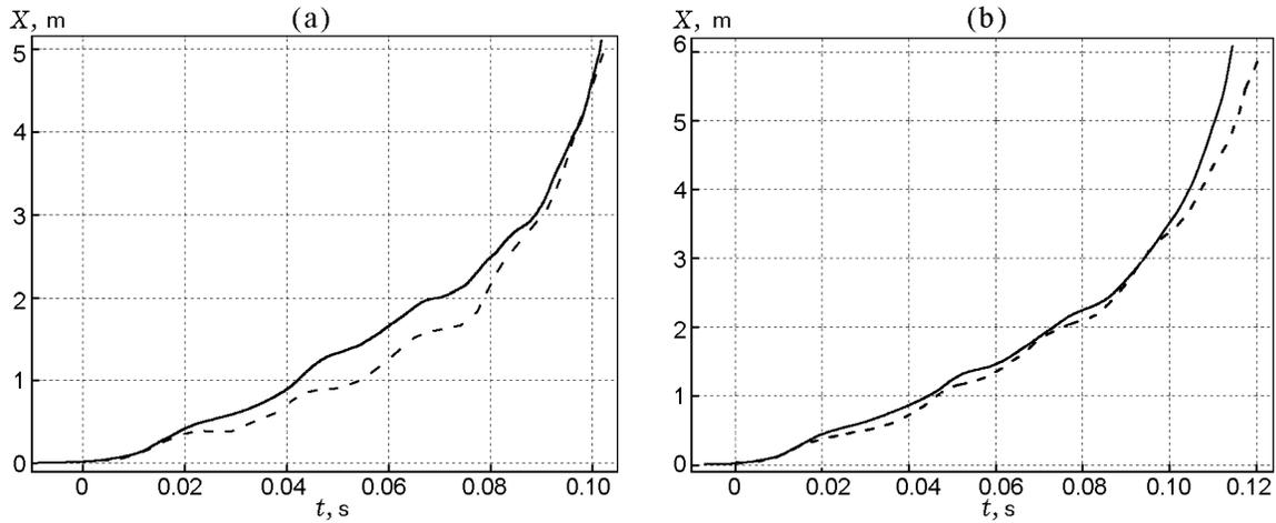
**Fig. 1.** Comparison of the calculated (solid curves) and experimental [15] (dashed curves) dependences of the distance covered by the flame in smooth tubes with a square cross section and length of 5.1 (a) and 6.1 m (b).
