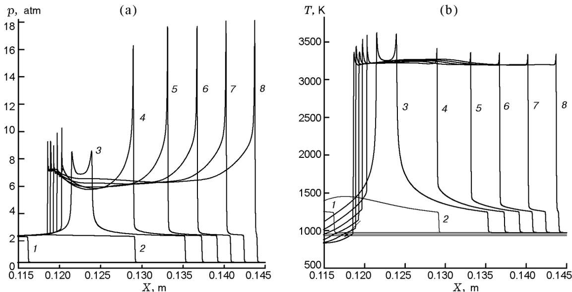
**Fig. 7.** Calculated profiles of pressure (a) and temperature (b) in the shock wave with preliminary thermal treatment of the mixture ( $C_5H_{12}:8O_2$ ):  $T_0 = 608$  K,  $p_0 = 0.42$  atm,  $t_i = 0.2$  s, and  $t - t_i = 98$  (1), 112 (2), 119 (3), 121 (4), 123 (5), 124.7 (6), 126.1 (7), and 128.1  $\mu$ s (8).
