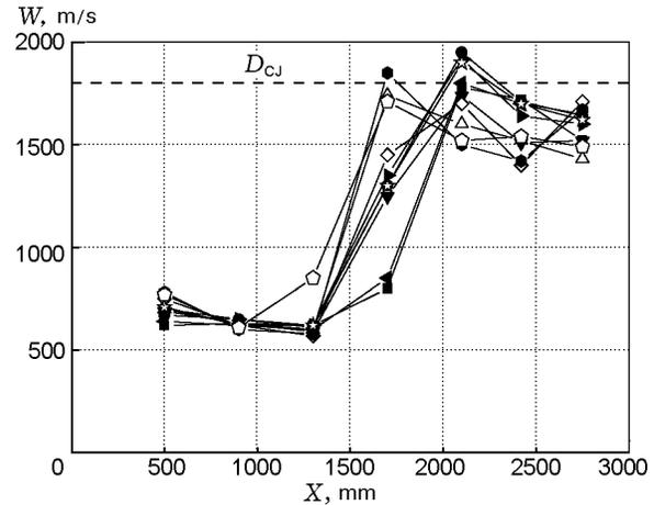
**Fig. 8.** Deflagration-to-detonation transition in a mixture of natural gas and air in ten cycles of operation of a pulsed-detonation burner with a frequency of 0.03 Hz with individual continuous supply of natural gas and air.
