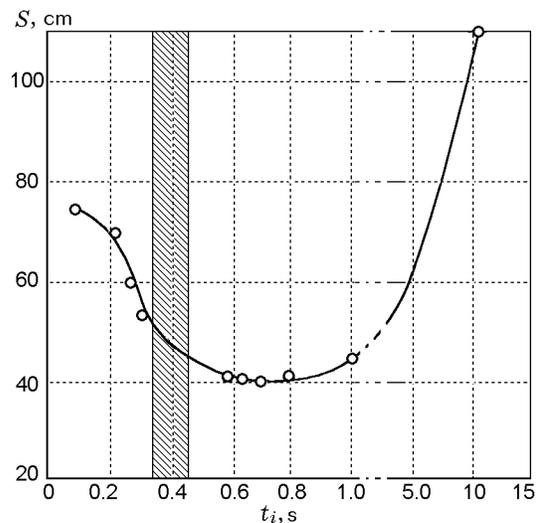
**Fig. 5.** Pre-detonation distance  $S$  versus the ignition delay  $t_i$  [3]:  $C_5H_{12}:8O_2$  mixture,  $T_0 = 608$  K and  $p_0 = 0.42$  atm; the hatched area shows the time of cold flame occurrence.
