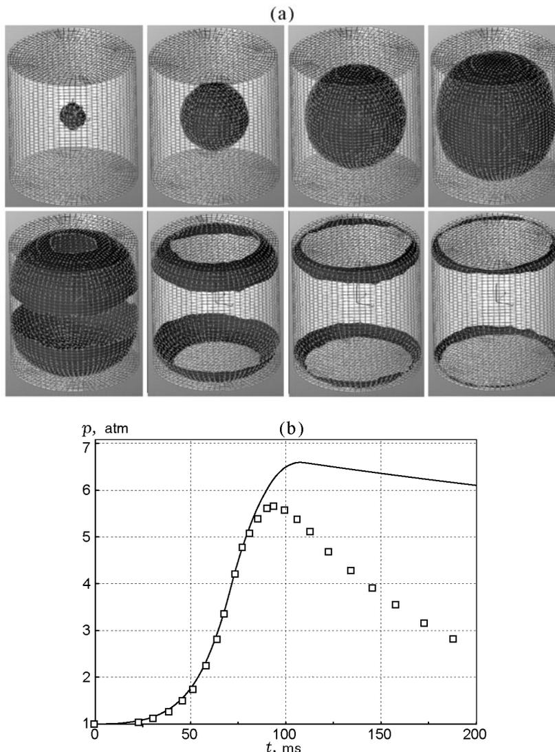
**Fig. 3.** Calculations of combustion of a propane–air mixture in a closed cylindrical vessel: (a) calculated positions of the flame front in the case of combustion of a rich ( $\phi = 1.1$ ) mixture for the following moments (from right to left):  $t = 5, 15, 25, 35, 45, 55, 65,$  and  $75$  ms; (b) calculated (curve) and measured [7] (points) dependences of pressure on time in the case of combustion of a lean ( $\phi = 0.8$ ) mixture.
