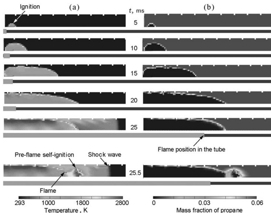
**Fig. 4.** Calculations of flame acceleration in a stoichiometric propane–air mixture until the instant of pre-flame self-ignition (only the upper half of the channel is shown).
