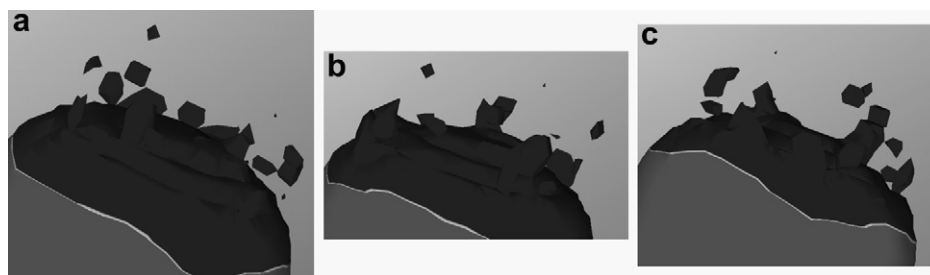
Fig. 8. Predicted snapshots of pre-flame autoignition at \sim 93 ms. Cylinder diameter is 172 mm.
