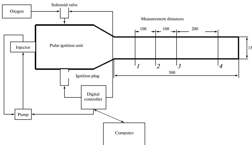
**Fig. 1.** Schematic of the demonstrator of the operation process in micro-PDRE: (1–4) ionization probes. The sizes are given in millimeters.
