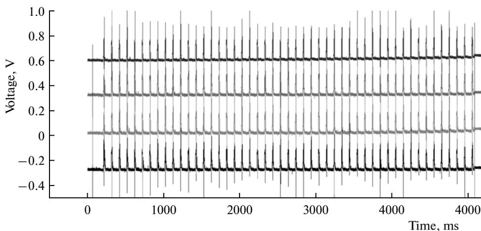
**Fig. 2.** Voltage signals from ionization probes 1–4 (from bottom to top) recorded for 5 s of operation of the micro-PDRE demonstrator (50 pulses at a repetition frequency of 10 Hz).
