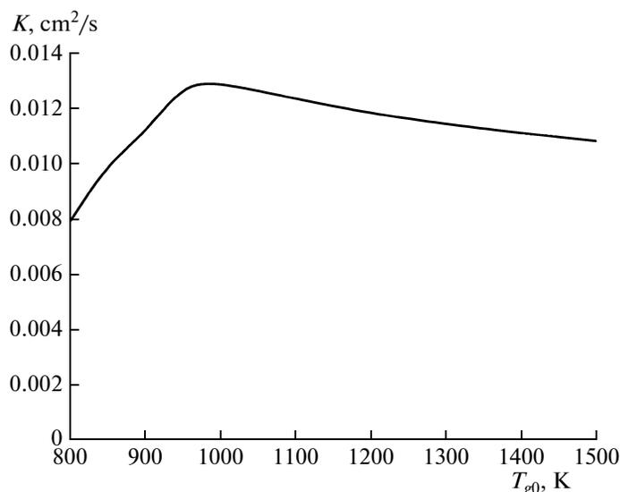
**Fig. 7.** Calculated dependence of the burning rate constant  $K$  for an  $n$ -heptane droplet on the initial temperature  $T_{g0}$  at  $d_0 = 60 \mu\text{m}$ ,  $P = 20 \text{ atm}$ , and  $\Phi = 1$ .
