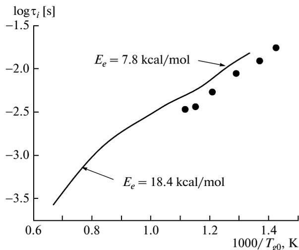
**Fig. 6.** Calculated dependence of the logarithm of the delay time of autoignition  $\log \tau_i$  of a droplet on the reciprocal temperature  $T_{g0}^{-1}$ :  $d_0 = 60 \mu\text{m}$ ,  $P = 20 \text{ atm}$ , and  $\Phi = 1$ . The symbols represent the experimental data from [28] for  $P = 21 \text{ atm}$ .
