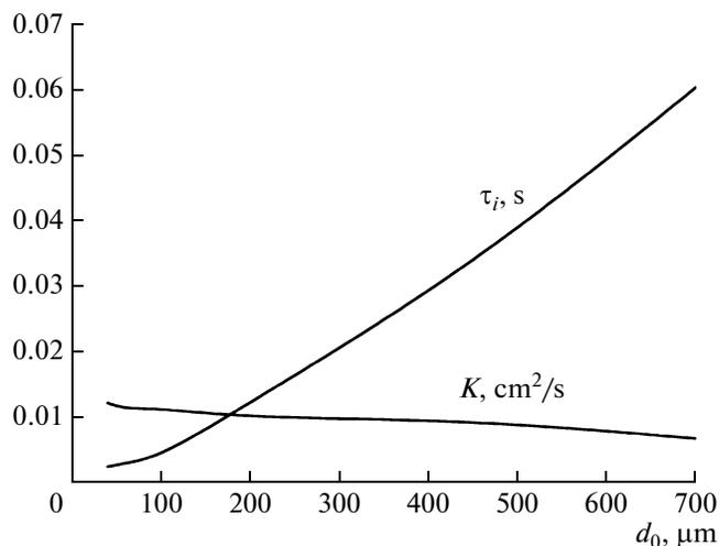
**Fig. 5.** Calculated dependences of the ignition delay time  $\tau_i$  and burning rate constant  $K$  of an *n*-heptane droplet on the initial droplet diameter  $d_0$  at  $T_{g0} = 1000 \text{ K}$ ,  $P = 20 \text{ atm}$ , and  $\Phi = 1$ .
