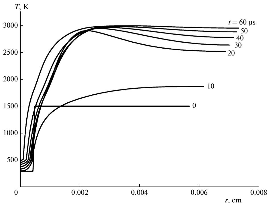
**Fig. 8.** Calculated spatial distribution of temperature over a droplet and around it at various moments of time at  $d_0 = 7.9 \mu\text{m}$ ,  $T_{g0} = 1500 \text{ K}$ ,  $P = 30 \text{ atm}$ ,  $\Phi = 1$ , and  $\Psi = 0.5$ .
