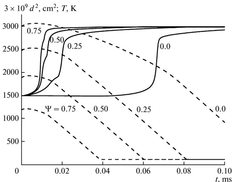
**Fig. 9.** Calculated time dependences of the maximum temperature  $T_{\max}$  of the gas (solid lines) and the squared droplet diameter  $d^2$  (dashed lines) at  $T_{g0} = 1500$  K,  $P = 30$  atm,  $\Phi = 1$ , and various degrees of pre-evaporation of droplets:  $\Psi = 0, 0.25, 0.50$ , and  $0.75$ .
