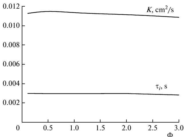
**Fig. 4.** Calculated dependences of the ignition delay time  $\tau_i$  and burning rate constant  $K$  of an *n*-heptane droplet on the fuel-to-oxidizer equivalence ratio  $\Phi$  for a gas–droplet suspension at  $d_0 = 60 \mu\text{m}$ ,  $T_{g0} = 1000 \text{ K}$ , and  $P = 20 \text{ atm}$ .
