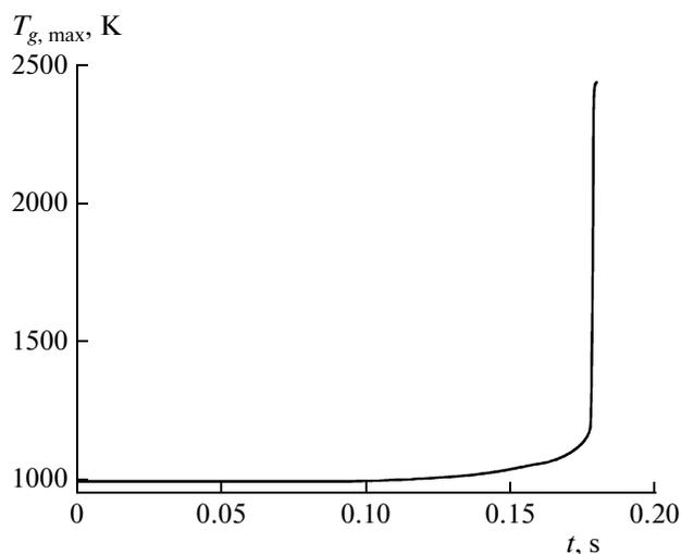
**Fig. 1.** Calculated time dependence of the maximum temperature  $T_{g, \max}$  of the gas around an *n*-heptane droplet during its autoignition:  $d_0 = 700 \mu\text{m}$ ,  $T_{g0} = 1000 \text{ K}$ ,  $P = 1 \text{ atm}$ , and  $\Phi = 0.46$ .
