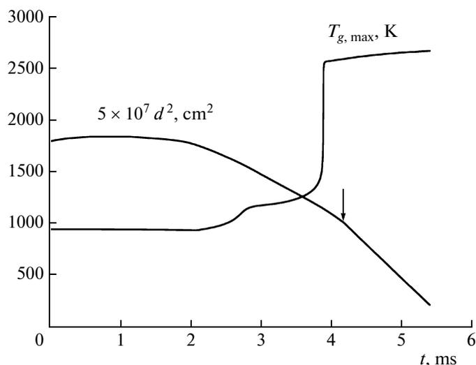
**Fig. 2.** Calculated time dependences of the maximum temperature  $T_{g, \max}$  of the gas around an *n*-heptane droplet and of the square of its diameter during autoignition:  $d_0 = 60 \mu\text{m}$ ,  $T_{g0} = 950 \text{ K}$ ,  $P = 20 \text{ atm}$ , and  $\Phi = 1$ .
