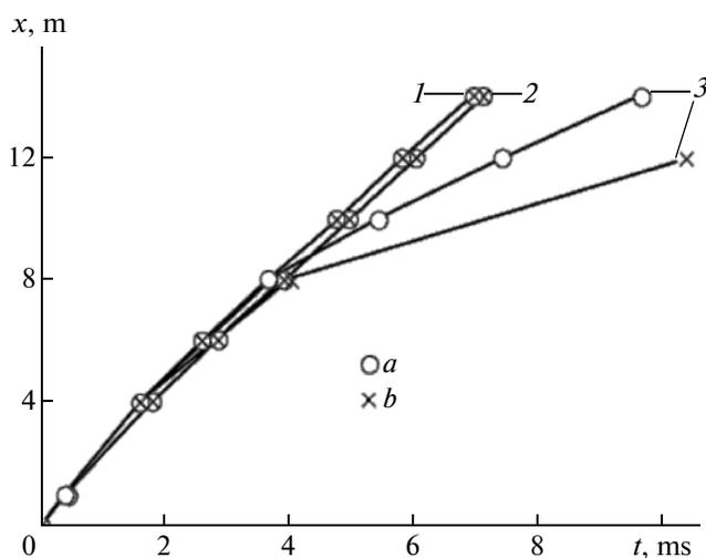
**Fig. 12.** Distance–time diagram for (a) shock wave and (b) reaction front propagation in 33.8% H<sub>2</sub>–air mixtures (1) without and (2, 3) with inhibitor in concentrations of (2) 2.0 and (3) 2.2 vol % [5].
