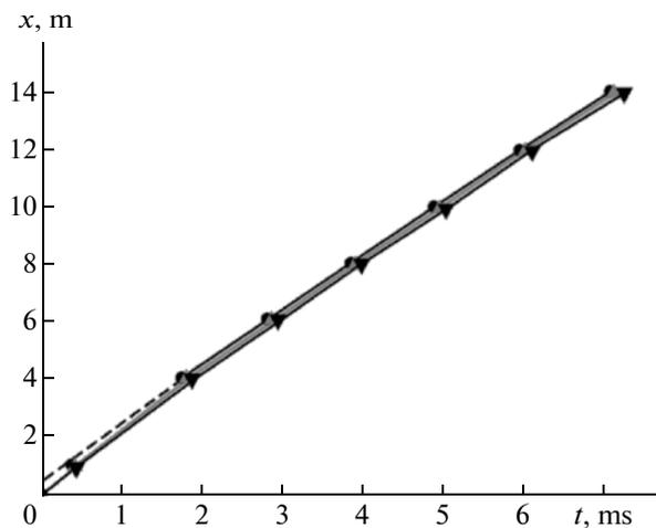
**Fig. 11.** Distance–time diagram for detonation propagation in a 33.8% H<sub>2</sub>–air mixture as measured in four experiments at the same initial conditions [5].
