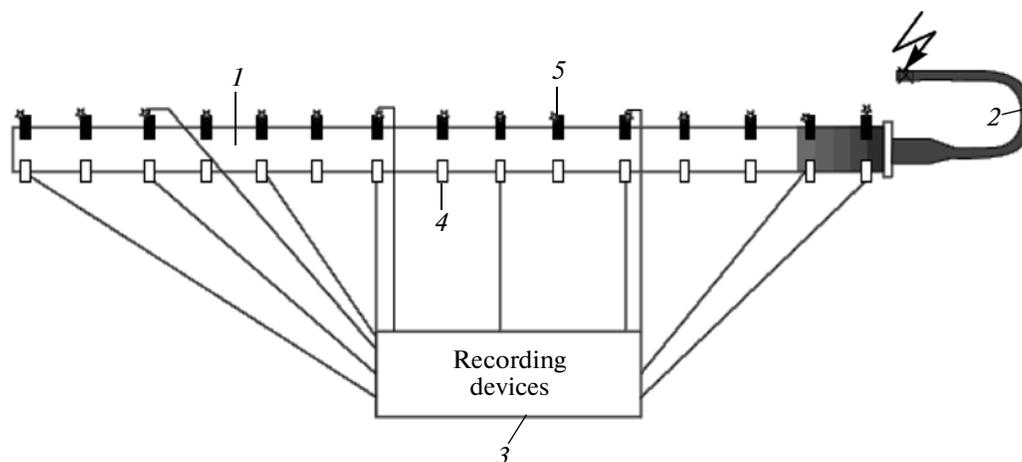
**Fig. 10.** Schematic of the experimental setup used in [5]: (1) detonation tube, (2) detonation initiation section, (3) recording devices, (4) pressure transducers, and (5) photodiodes.
