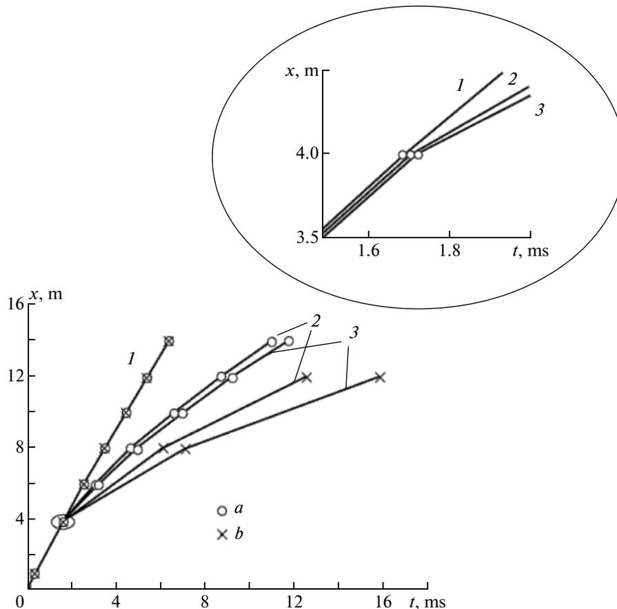
**Fig. 13.** Distance–time diagram for (a) shock wave and (b) reaction front propagation in 45% H<sub>2</sub>–air mixtures (1) without and (2, 3) with inhibitors: (2) 2.5 vol % propene and (3) 2.5 vol % isobutene [5].
