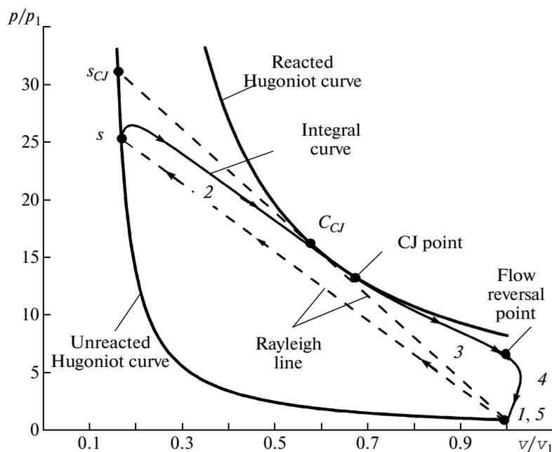
Fig. 2. Changes in the state of the gas in the detonation wave illustrated in the pressure–specific volume plane.
