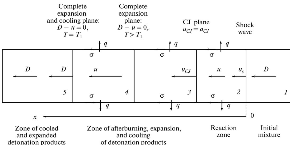
Fig. 1. Structure of a steady detonation wave.
