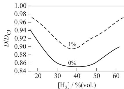
**Figure 8** Predicted dependence of detonation velocity deficit on hydrogen concentration in H<sub>2</sub>–air mixture. Curve “0%” corresponds to the mixture without inhibitor, curve “1%” corresponds to the mixture with 1% propene. Initial parameters:  $p_1 = 0.1$  MPa and  $T_1 = 298$  K
