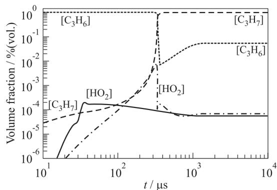
**Figure 5** Predicted time histories of  $C_3H_6$ ,  $C_3H_7$ , and  $HO_2$  concentrations at autoignition of 29.6%  $H_2$  + 70.4% air (broken curves) and 29.6%  $H_2$  + 1.0%  $C_3H_6$  + 69.4% air (solid curve) mixtures at  $p_1 = 0.1$  MPa and  $T_1 = 1200$  K
