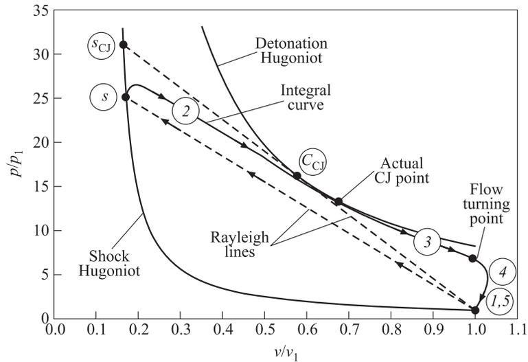
**Figure 2** Variation of mixture state in the detonation wave at the pressure–specific volume plane
