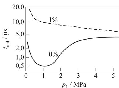
**Figure 3** Predicted ignition delay time as a function of initial pressure for the stoichiometric  $H_2 + air$  mixture with 1% (vol.) (curve 1%) and without (curve 0%) propene additive at initial temperature  $T_1 = 1200$  K
