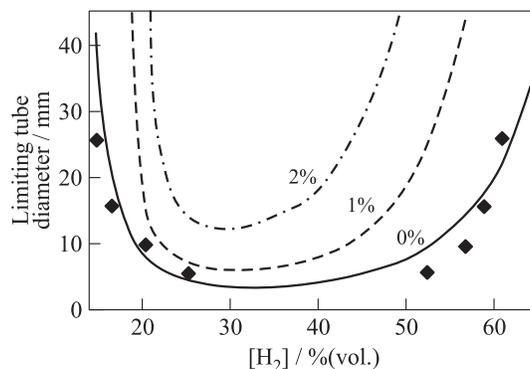
**Figure 6** Limiting tube diameter as a function of hydrogen concentration in hydrogen–air mixture. Curves “0%,” “1%,” and “2%” correspond to different percentage (vol.) of propene in the mixture. Initial parameters:  $p_1 = 0.1$  MPa and  $T_1 = 298$  K. Diamonds show the results of direct experiments [23] for pure hydrogen–air mixtures
