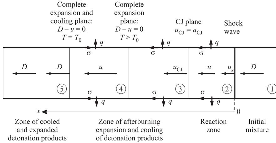
**Figure 1** Structure of 1D steady-state detonation wave
