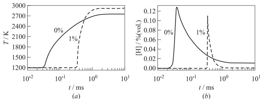
**Figure 4** Predicted time histories of temperature (a) and atomic hydrogen concentration (b) for autoignition of 29.6%  $H_2$  + 70.4% air (curve “0%”) and 29.6%  $H_2$  + 1.0%  $C_3H_6$  + 69.4% air (curve “1%”) at  $p_1 = 0.1$  MPa and  $T_1 = 1200$  K
