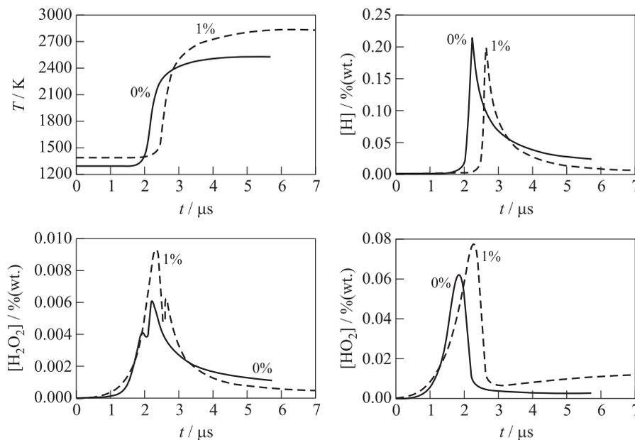
**Figure 7** Predicted time histories of temperature and mass fractions of H, HO<sub>2</sub>, and H<sub>2</sub>O<sub>2</sub> in hydrogen–air–inhibitor detonations. Curves “0%” correspond to 22% (vol.) H<sub>2</sub> + 78% (vol.) air mixture. Curves “1%” correspond to 22% (vol.) H<sub>2</sub> + 1% (vol.) C<sub>3</sub>H<sub>6</sub> + 77% (vol.) air mixture. Initial parameters:  $p_1 = 0.1$  MPa and  $T_1 = 298$  K
