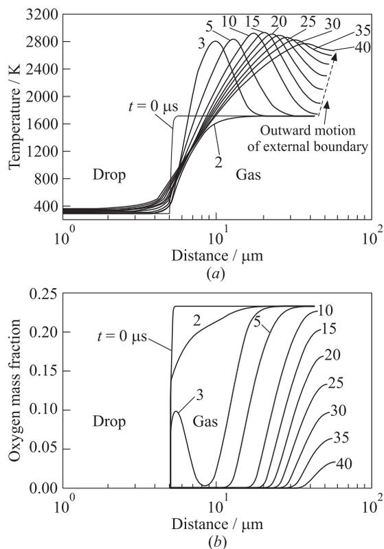
**Figure 2** Predicted time histories of temperature (a) and oxygen mass fraction (b) around an *n*-heptane drop in the micromist for the conditions relevant to Fig. 1. Numbers correspond to different time instants (in microseconds) counted from shock compression ( $t = 0$ ). Ignition occurs at approximately  $3 \mu\text{s}$
