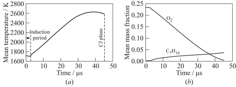
**Figure 1** Predicted evolution of temperature (a) and mass fractions of *n*-heptane and oxygen (b) in the heterogeneous detonation wave propagating in the monodisperse *n*-heptane suspensions with the initial drop radius of 50  $\mu\text{m}$  (micromist drop radius of 5  $\mu\text{m}$ ) at 1 bar, 293 K, and  $\Phi \approx 2.5$  ( $\eta_d = 0.2 \text{ kg/m}^3$ )
