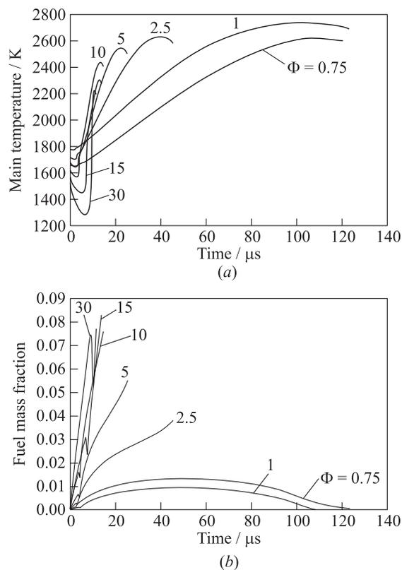
**Figure 3** Time histories of temperature (a) and fuel mass fraction (b) in self-sustained detonation waves propagating in monodisperse *n*-heptane suspensions with the initial drop radius  $50 \mu\text{m}$  (micromist drop radius  $5 \mu\text{m}$ ) at different equivalence ratios. Initial pressure is 1 bar, initial gas temperature is 293 K, initial liquid temperature is 293 K
