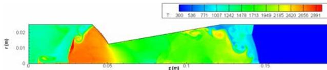
Figure 3 – Detonation initiation failure in a tube with parabolic contraction and smooth conic expansion at  $M = 2.7$ ,  $\varphi = 50^\circ$ ,  $BR = 0.75$ . Predicted field of temperature (in K). Time  $137 \mu s$ .
