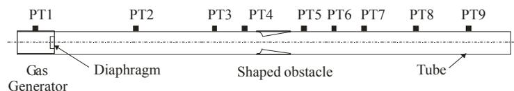
Figure 5 – Experimental setup.
