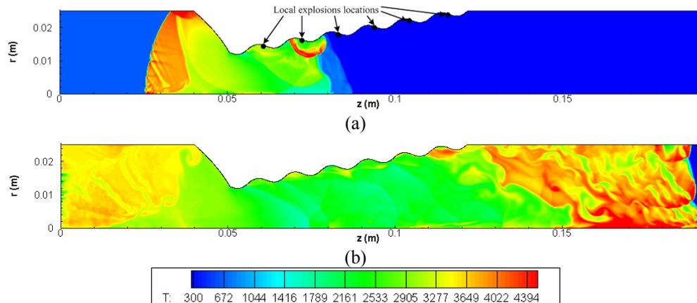
Figure 4 – Detonation initiation in a tube with parabolic contraction and sinusoidal conic expansion under conditions similar to those in Fig. 3. Predicted fields of temperature (in K). The upper snapshot corresponds to time 90  $\mu$ s, the lower to 140  $\mu$ s.
