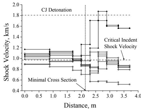
Figure 6 – Mean SW velocity at different measuring segments vs. distance.
