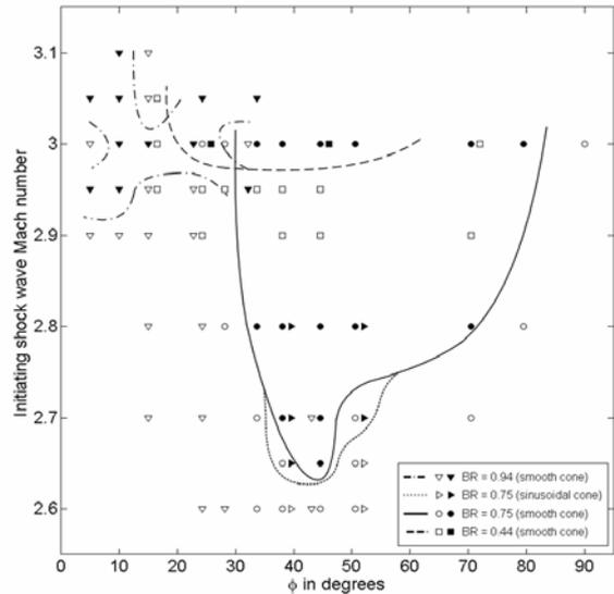
Figure 2 – “Detonation curves”: open symbols – SDT “no go”, closed symbols – SDT “go” conditions.
