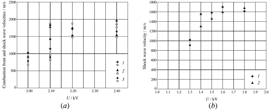
**Figure 14:** Measured shock wave (solid symbols) and flame front (open symbols) velocities as a function of discharge voltage for *n*-hexane sprays in air in tubes of different inner diameter: 51 mm (a) and 28 mm (b). Numbers 1 to 3 denote the measuring stations located at 500, 900, and 1300 mm (a) and 125, 525, and 925 mm (b) from the discharge [16, 17]
