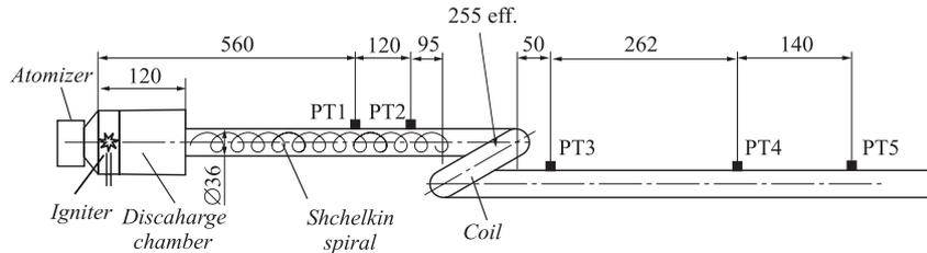
**Figure 21:** Schematic of an explosion tube 36 mm in diameter with a coil
