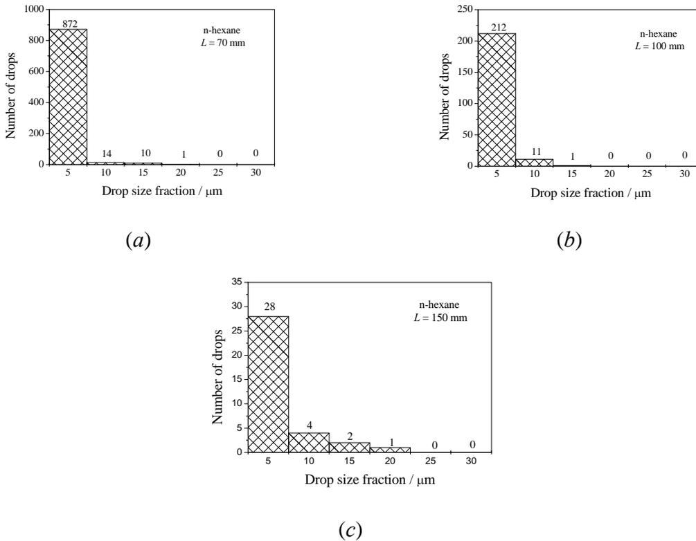
**Figure 7:** Measured drop size distributions in *n*-hexane spray at  $L = 70$  mm (a), 100 (b), and 150 mm (c). Drop size fractions plotted along  $X$ -axes are chosen divisible to  $5 \mu\text{m}$ . Size fraction of  $5 \mu\text{m}$  corresponds to drops of size less than  $5 \mu\text{m}$ , size fraction  $10 \mu\text{m}$  corresponds to drops with size exceeding  $5 \mu\text{m}$  and less than  $10 \mu\text{m}$ , etc.
