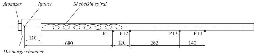
**Figure 19:** Schematic of a straight explosion tube 36 mm in diameter with air-assist atomizer, igniter, discharge chamber, Shchelkin spiral, and pressure transducers PT1 to PT4
