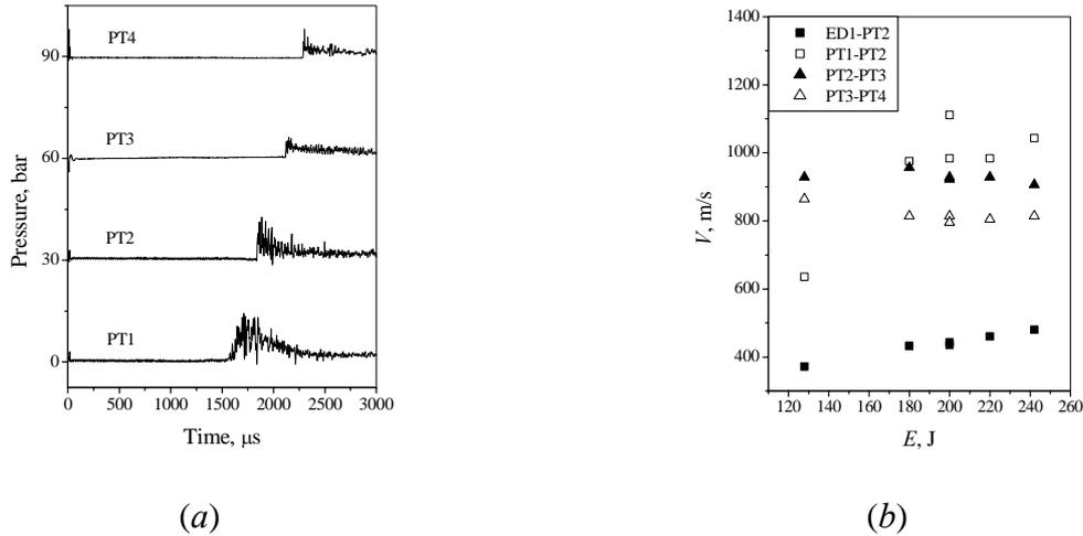
**Figure 20:** Pressure profiles recorded by transducers PT1–PT4 in an experiment with an ignition energy of  $E = 128$  J (a), and the measured shock wave velocity in a drop *n*-hexane–air mixture over different measurement segments vs. ignition energy (b)
