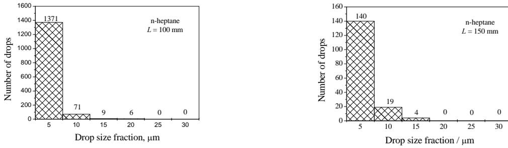
**Figure 8:** Measured drop size distributions in *n*-heptane spray at  $L = 100$  mm (a) and 150 mm (b)
