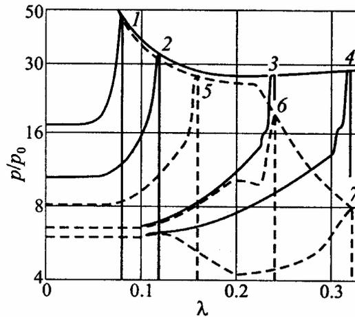
**Figure 1:** Predicted explosion dynamics under supercritical (solid curves) and subcritical (dashed curves) initiation of detonation in gas–drop suspension;  $\lambda = r / r^0$  is the dimensionless distance; numbers correspond to different successive time instants [7]
