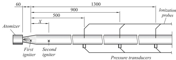
**Figure 15:** Schematic of the test tube with air-assist atomizer, two igniters, line of pressure transducers, and line of ionization probes;  $X$  is the distance between successively triggered igniters
