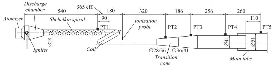
**Figure 23:** Schematic of an explosion tube 28 mm in diameter with a coil and a transition section to a tube 51 mm in diameter
