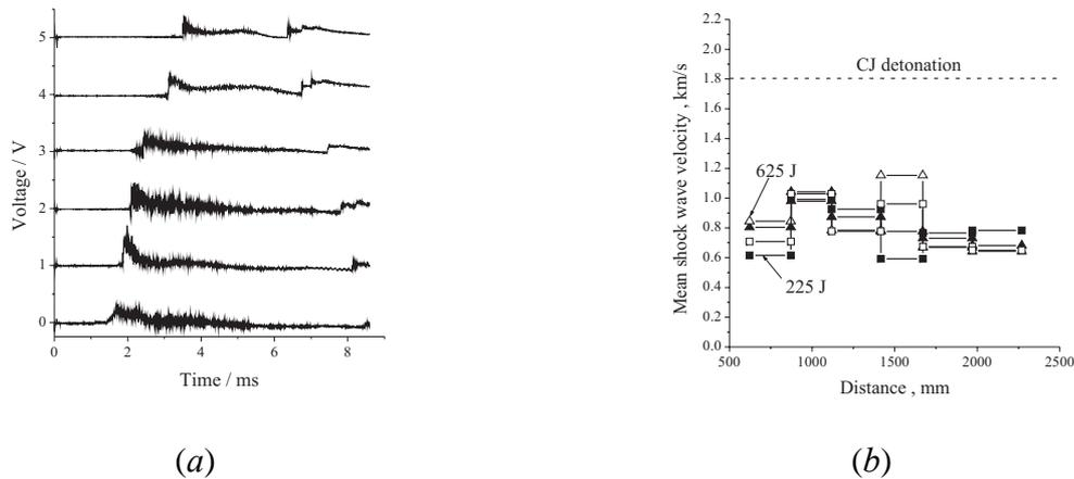
**Figure 26:** Pressure profiles recorded by transducers PT1–PT6 in an experiment with an ignition energy of  $E = 225$  J (a), and the measured shock wave velocities in a two-phase mixture of aviation kerosene with air over different measurement segments at different ignition energies (b)
