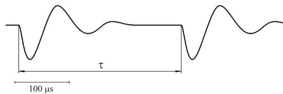
**Figure 16:** Discharge current in a two-discharge circuit measured by the Rogowsky coil mounted on the high-voltage cable. The signal was obtained at voltage 2500 V and rated capacitance 300  $\mu$ F for each discharge. The second igniter was triggered 300  $\mu$ s after the first igniter
