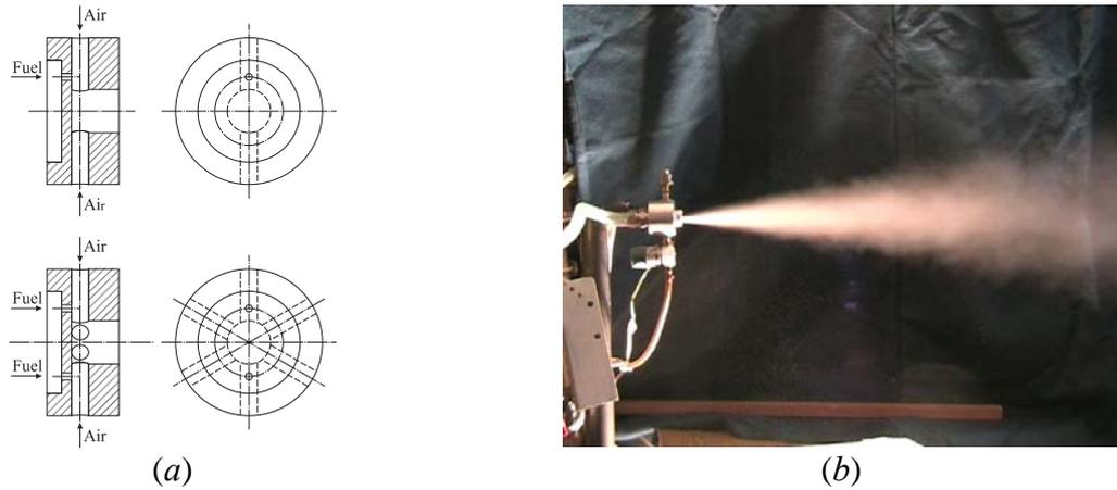
**Figure 4:** Air-assist atomizers (a) and spray image (b). Air is supplied either via 2 or 6 radial channels. Liquid fuel is supplied via one or two axial channels into the air channel
