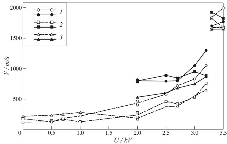
**Figure 9:** Measured shock wave (solid curves) and flame front (dashed curves) velocities vs. igniter voltage (*n*-hexane) at different measuring segments (1 to 3). Due to poor accuracy of pressure measurements at low ignition energies, measurements of shock wave velocity were performed beginning from the voltage of 2000 V
