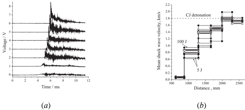
**Figure 27:** Pressure profiles recorded by transducers PT1–PT7 in an experiment with an ignition energy of  $E = 5 \text{ J}$  (a), and the measured shock wave velocities in a two-phase mixture of aviation kerosene with air over different measurement segments at different ignition energies (b)
