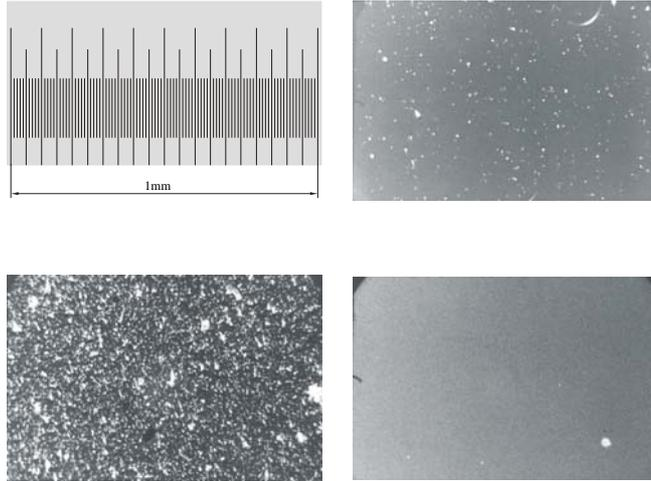
**Figure 6:** Photographs of *n*-hexane spray signature on the target rod surface: Upper left – scale of the photographs; bottom left – spray signature at distance 70 mm from the nozzle; upper right – spray signature at distance 100 mm from the nozzle; bottom right – spray signature at distance 150 mm from the nozzle
