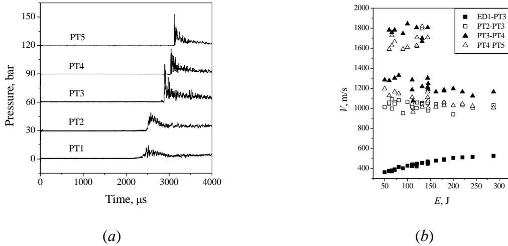
**Figure 22:** Pressure profiles recorded by transducers PT1–PT5 in an experiment with an ignition energy of  $E = 60$  J (a), and the measured shock wave velocity in a drop  $n$ -hexane–air mixture over different measurement segments vs. ignition energy (b).
