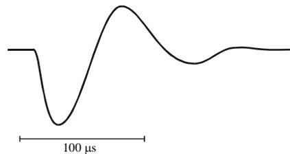
**Figure 3:** Discharge current measured by the Rogowsky coil mounted on the high-voltage cable. The signal was obtained at voltage 2500 V and rated capacitance 300  $\mu\text{F}$ . The shape of current is close to sin wave with the oscillation period of  $100 \pm 10 \mu\text{s}$
