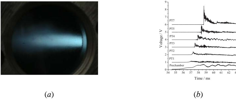
**Figure 28:** Flame jet issuing from the igniter nozzle at ignition energy of 100 mJ (a) and pressure profiles recorded by transducers PT1–PT7 and a transducer located in the prechamber for the experiment with liquid gasoline A-80 – air mixture at ignition energy of  $E = 100 \text{ mJ}$  (b)
