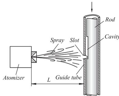
**Figure 5:** Schematic of the express-method used for drop size measurements. The measurements were performed by means of fast intrusion of thin target rods through the spray across its centerline attributed to drop sizes. The plates were examined with the use of optical microscope and drop size distributions were obtained.
