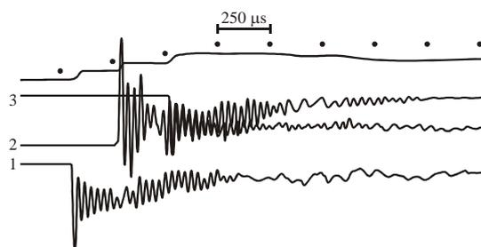
**Figure 11:** Records of ionization current (upper beam with time markers) and pressure at measuring stations 1, 2, and 3 at the ignition energy of 3324 J in the *n*-hexane spray. The pressure and ionization gauge records at the corresponding measuring stations indicate simultaneous arrival of a shock wave and flame front
