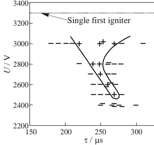
**Figure 18:** Detonation initiation energy (in terms of voltage  $U$  applied to the high-voltage blocks of two igniters with similar capacity of  $300 \mu\text{F}$ ) vs. the delay time  $\tau$  of triggering the second igniter (counted from activation of first igniter) [14, 15]
