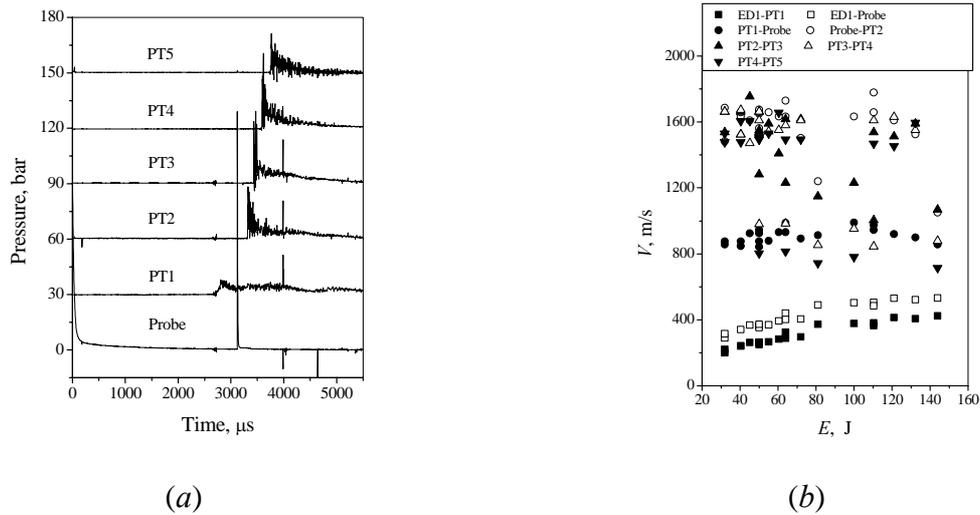
**Figure 24:** Pressure profiles recorded by transducers PT1–PT5 in an experiment with an ignition energy of  $E = 32$  J (a), and the measured shock wave velocity in a drop *n*-hexane–air mixture over different measurement segments vs. ignition energy (b).
