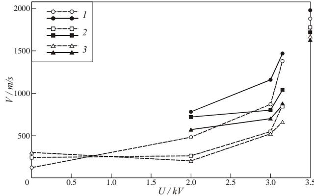
**Figure 13:** Measured shock wave (solid curves) and flame front (dashed curves) velocities vs. igniter voltage for the *n*-heptane spray at different measuring segments (1 to 3). Due to poor accuracy of pressure measurements at low ignition energies, the measurements of the shock wave velocity were performed started from the voltage of 2000 V
