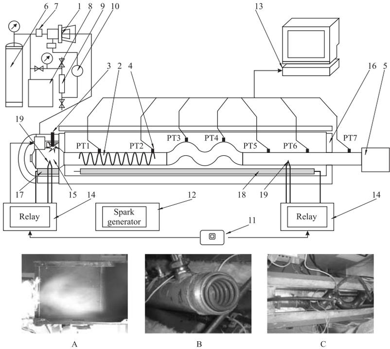
**Figure 25:** Schematic of the experimental setup with a kerosene prevaporizer (A), Shchelkin spiral (B), and 2-coil tube section enhancing fast DDT (C)
