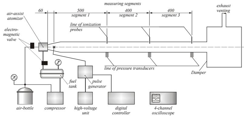
**Figure 2:** Sketch of the experimental setup [14, 15]
