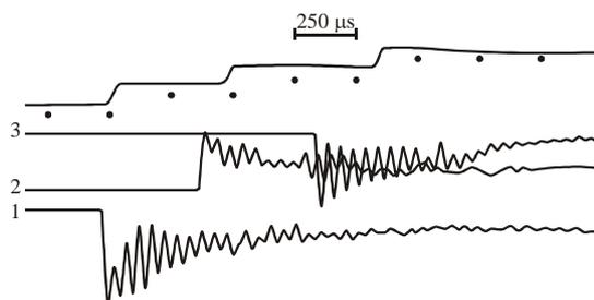
**Figure 12:** Records of ionization current (upper beam with time markers) and pressure at measuring stations 1, 2, and 3 at the ignition energy of 3324 J in the *n*-heptane spray. The comparison of pressure and ionization gauge records at the corresponding measuring stations indicates that flame lags behind the lead shock wave in this run
