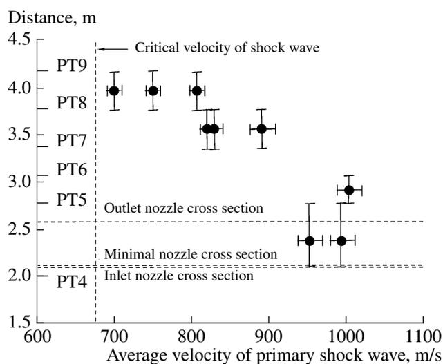
Fig. 4. Detonation run-up distance versus average velocity of the primary shock wave at the nozzle inlet.
