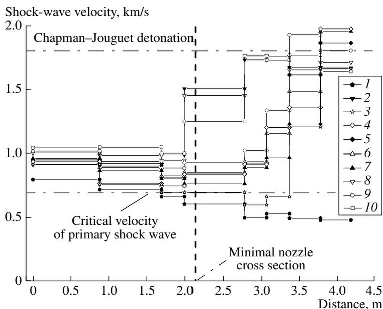
**Fig. 2.** Average velocity of the leading shock front versus travelled distance in various measuring segments in 10 representative experiments.
