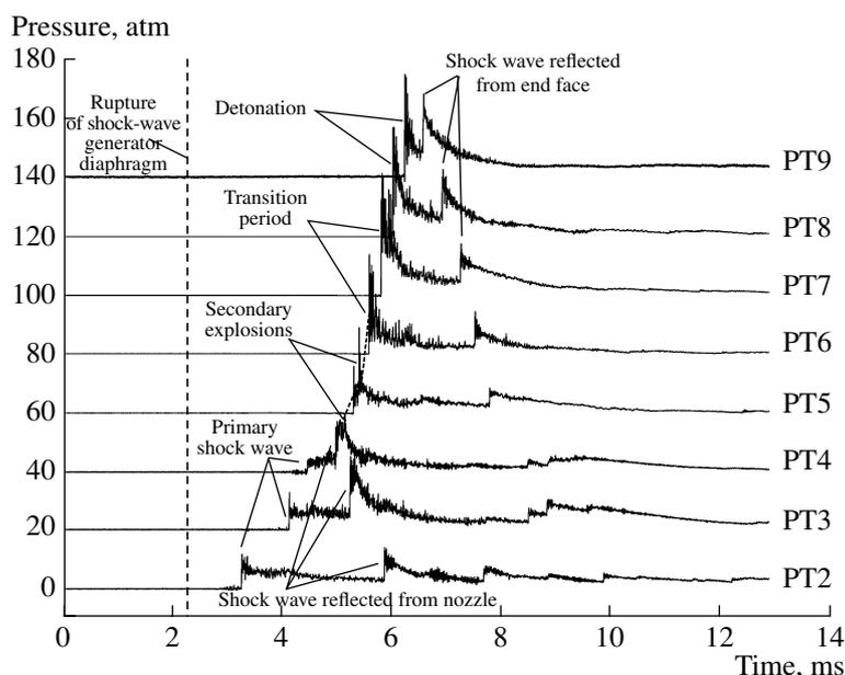
**Fig. 3.** Pressure records of transducers PT2–PT9 in experiment 9 with identification of wave phenomena.
