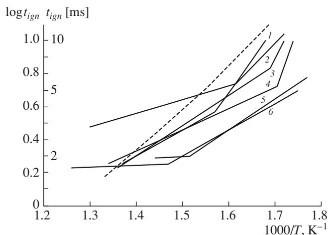
**Fig. 4.** Comparison of the temperature dependences of the calculated and experimental [25] self-ignition delay times for various fuels at pressure 2.5 MPa. The dashed line corresponds to *n*-tetradecane drops with the initial diameter  $D_0 = 20 \mu\text{m}$ . Solid curves correspond to motor fuels with different cetane numbers (CN) and different sprayers (1 and 2). CN/sprayer: (1) 49/1, (2) 50/1, (3) 49/2, (4) 50/2, (5) 70/2, and (6) 62/2.
