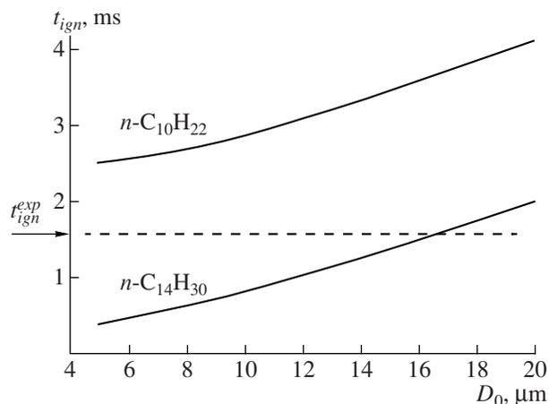
**Fig. 5.** Comparison of calculated self-ignition delay times with delay times measured in a real diesel engine. Calculations were performed for stoichiometric ( $\Phi = 1.0$ ) gas suspensions of *n*-decane (the upper curve) and *n*-tetradecane (the lower curve) drops with different initial diameters at air temperature and pressure 800 K and 4 MPa, respectively.
