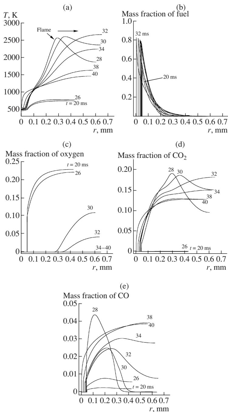
**Fig. 6.** Calculated spatial distributions of (a) temperature and mass fractions of (b) fuel vapor, (c) oxygen, (d)  $\text{CO}_2$ , and (e) CO in the self-ignition of an *n*-decane drop with the initial diameter  $100\ \mu\text{m}$  in a uniform gas suspension of drops with  $\Phi = 2$  at pressure 2 MPa and air temperature 800 K.
