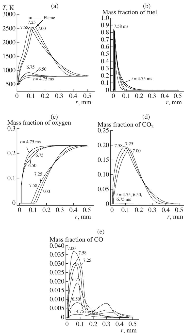
**Fig. 7.** Calculated spatial distributions of (a) temperature and mass fractions of (b) fuel vapor, (c) oxygen, (d)  $\text{CO}_2$ , and (e) CO in the self-ignition of an *n*-decane drop with the initial diameter  $40\ \mu\text{m}$  in a uniform gas suspension of drops with  $\Phi = 0.1$  at pressure 2 MPa and air temperature 800 K.
