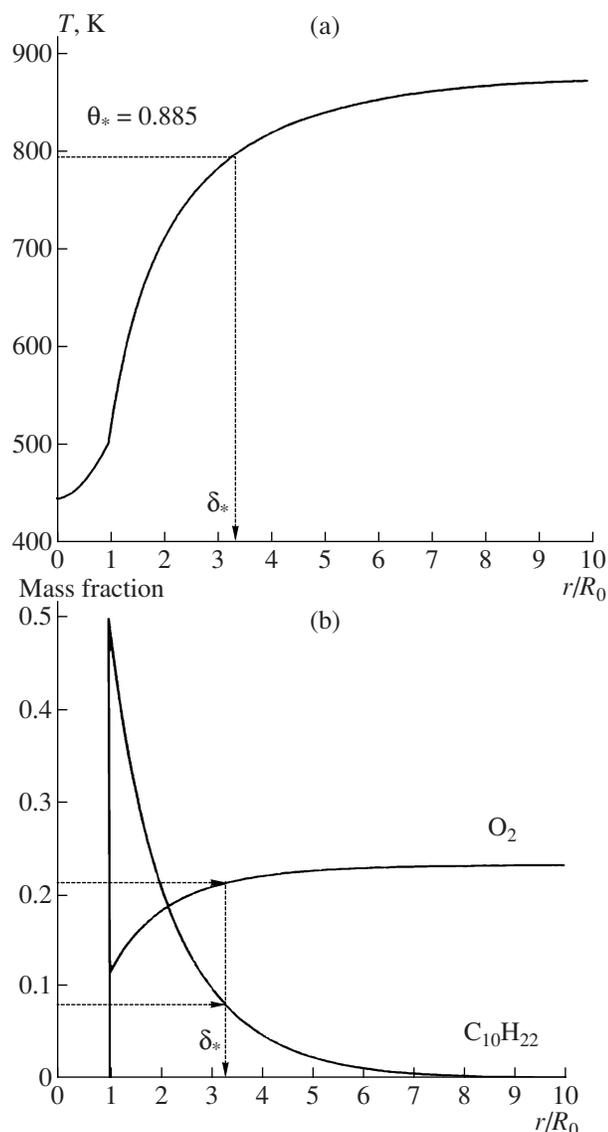
**Fig. 8.** Determination of (a) reduced temperature and (b) local equivalence ratio in a vapor-gas mixture at the reduced self-ignition radius.
