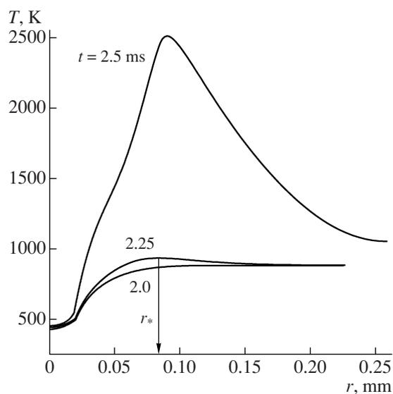
**Fig. 2.** Calculated spatial distributions of temperature in the self-ignition of an *n*-decane drop in air. Initial parameters:  $D_0 = 40 \mu\text{m}$ ,  $T_0 = 300 \text{ K}$ ,  $T_{g0} = 900 \text{ K}$ ,  $p = 2 \text{ MPa}$ , and  $\Phi = 1.0$ .
