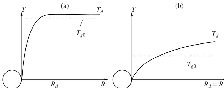
Fig. 12. Scheme of temperature profiles in the vicinity of a drop at (a)  $t < t_d$  and (b)  $t > t_d$ .
