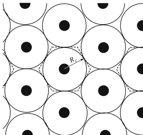
**Fig. 1.** Definition of an elementary grid cell in a uniform monodisperse gas suspension of drops [19, 20]. Solid circles are drops. Circles around drops characterize the depth of the penetration of diffusion fluxes. The dashed line bounds the elementary cell through the surface of which there are no energy and mass fluxes;  $R_c$  is the characteristic size of the cell.
