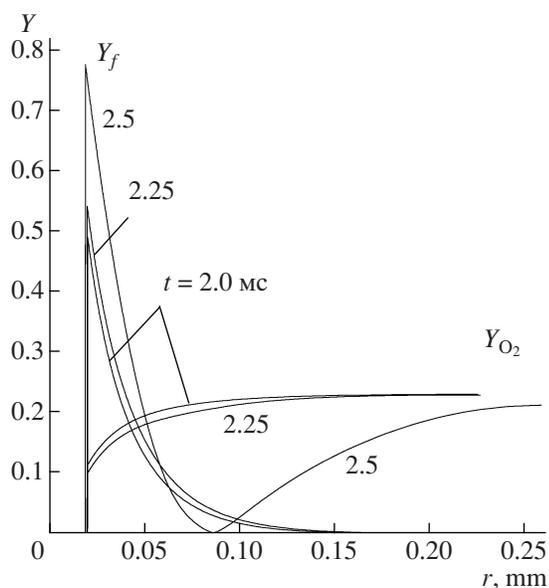
**Fig. 3.** Calculated spatial distributions of the mass fractions of oxygen and fuel vapor in the self-ignition of an *n*-decane drop in air. Initial parameters:  $D_0 = 40 \mu\text{m}$ ,  $T_0 = 300 \text{ K}$ ,  $T_{g0} = 900 \text{ K}$ ,  $p = 2 \text{ MPa}$ , and  $\Phi = 1.0$ .
