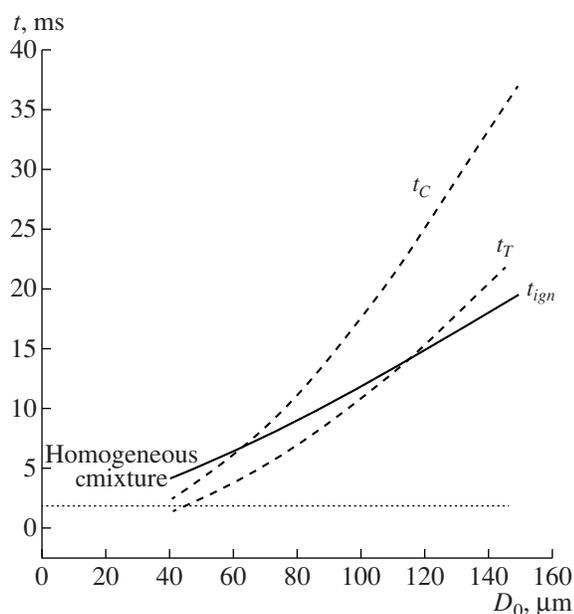
**Fig. 11.** Calculated dependences of self-ignition delay times  $t_{ign}$ ,  $t_T$ , and  $t_C$  on the initial diameter of  $n$ -decane drops at  $T_{g0} = 850$  K and  $p = 2$  MPa.
