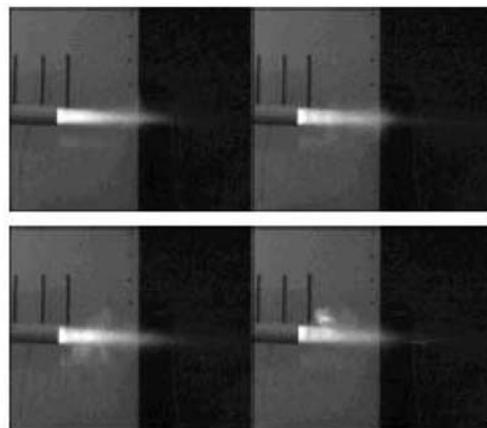
**Fig. 6.** Images of periodic supersonic flows of detonation products during operation of PDE demonstrator.
