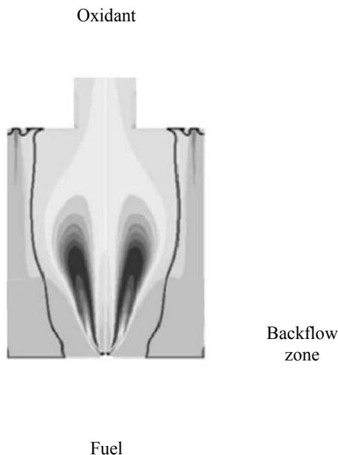
Fig. 1. Scheme of the organization of flameless combustion [2].
