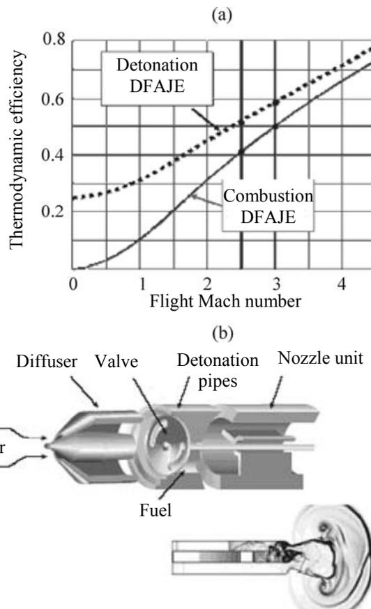
**Fig. 5.** (a) Advantages of detonative fuel combustion and (b) scheme of pulse detonative engine for aircrafts.
