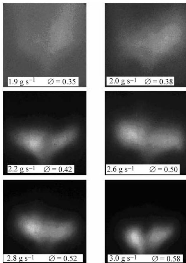
Fig. 2. OH\* chemiluminescence images at 310 nm in propane-air mixtures with different fuel excess factors  $\Phi$  [2].
