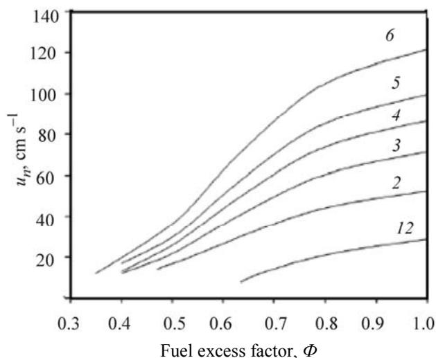
**Fig. 4.** Dependences of rate  $u_n$  on fuel excess factor  $\Phi$  for flame propagation in: (1) cold-wall hollow pipe (critical conditions:  $\Phi^* = 0.635$ ,  $u_n = 7.85 \text{ cm s}^{-1}$ ); (2) porous-wall pipe without heating; (3–6) porous-wall pipe with a local outer heating [(3)  $0.01\Theta_{\text{max}}$ , (4)  $0.02\Theta_{\text{max}}$ , (5)  $0.03\Theta_{\text{max}}$ , (6)  $0.05\Theta_{\text{max}}$ ].
