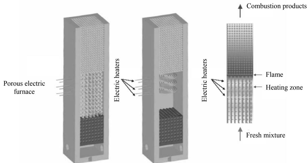
Fig. 3. Scheme of a porous electric furnace with additional heat supply to the flame heating zone by means of electric heaters.
