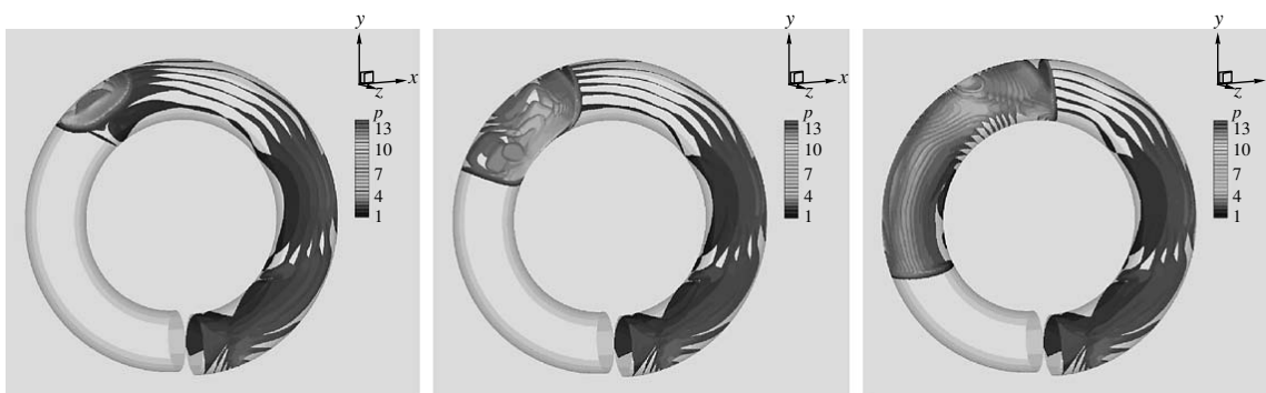
Fig. 7. Calculated dynamics of static pressure isosurfaces (in MPa) during a deflagration-to-detonation transition in a tube coil 28 mm in diameter (the first configuration); the Mach number of the primary shock wave M = 3.9 .
