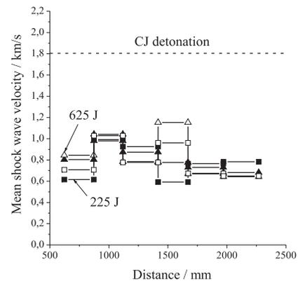
Figure 6: Measured mean shock wave velocities as a function of distance from the igniter in 4 runs with the ignition energy varied from 225 to 625 J
