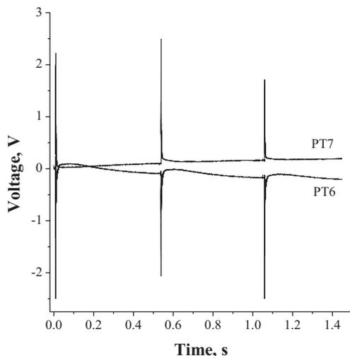
Figure 9: Records of pressure transducers PT6 and PT7 in three successive detonation pulses at the operation frequency of about 2 Hz
