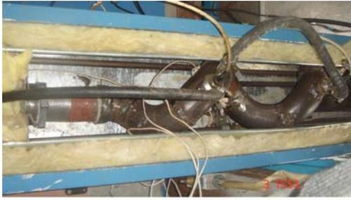
Figure 4: The curved tube segment in the thermostat
