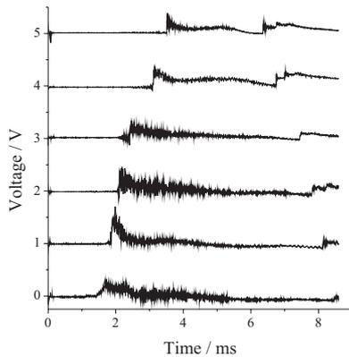
Figure 5: Pressure records in the run with igniter energy of 225 J
