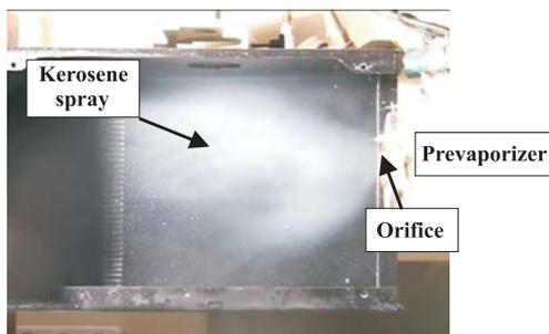
Figure 2: Visualization of kerosene spray exhasting from the prevaporizer orifice (right) at prevaporizer wall temperature 90 °C
