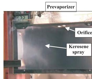
Figure 3: Visualization of kerosene spray exhasting from the prevaporizer orifice (top) at prevaporizer wall temperature of 225 °C
