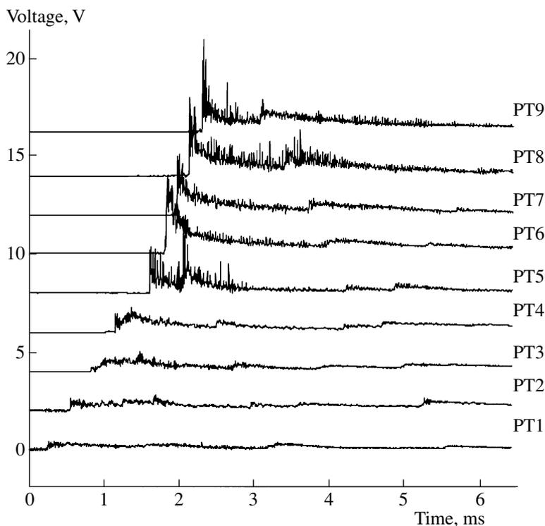
**Fig. 3.** Records of pressure transducers PT1–PT9 in the run with detonation initiation downstream of the second U-bend in a tube 51 mm in diameter.
