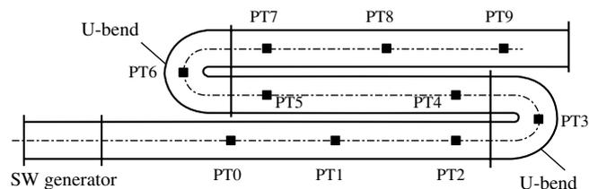
Fig. 1. Tube with two U-bends, an SW generator, and pressure transducers PT0–PT9. PT0 is the triggering transducer.
