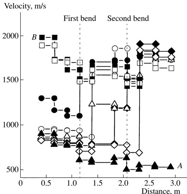
**Fig. 2.** Mean SW velocity over different measuring segments in a tube 51 mm in diameter with two U-bends. Symbols are used for simplifying curve identification. The vertical dashed lines correspond to the location of pressure transducers PT3 and PT6 in the U-bends.
