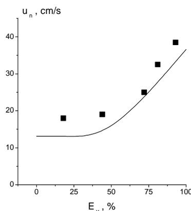
**Fig. 5:** Predicted (curve) and measured ([4]) laminar flame velocities in *iso*-octane drop suspensions in air as a function of the prevaporization degree,  $E_v$ .  $\phi=1$ ,  $T_0 = 293$  K,  $p_0 = 0.1$  MPa. At  $E_v = 0$ ,  $d_{s0} = 100 \mu\text{m}$
