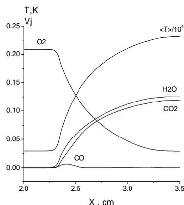
**Fig. 4:** Predicted spatial distributions of temperature and molar fractions of main species in the laminar flame propagating in *iso*-octane drop suspension in air.  $d_{s0} = 100$   $\mu\text{m}$ .  $\phi = 1$ ,  $T_0 = 293$  K,  $p_0 = 0.1$  MPa
