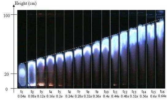
Fig. 2: Sequence of flame propagation in the suspension of *iso*-octane drops in air
