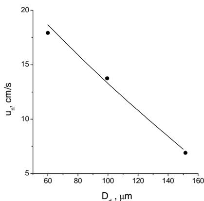
**Fig. 3:** Comparison of predicted (line) and measured (symbols, [4]) laminar flame velocities in *iso*-octane drop suspensions in air as a function of initial drop diameter.  $\phi = 1$ ,  $T_0 = 293$  K,  $p_0 = 0.1$  MPa
