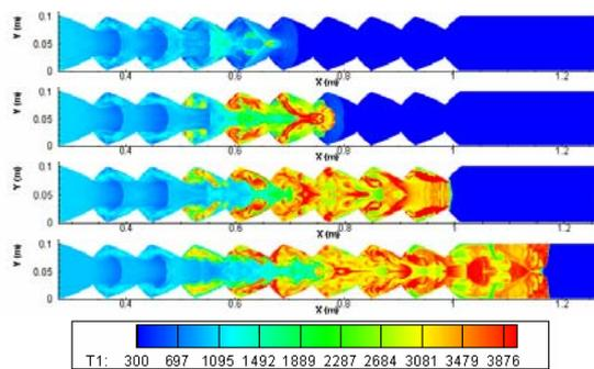
**Fig. 3:** Snapshots of temperature fields at SDT in the channel with regular parabolic obstacles. The upper snapshot corresponds to  $480 \mu\text{s}$ . Other snapshots are plotted with the time interval of  $100 \mu\text{s}$
