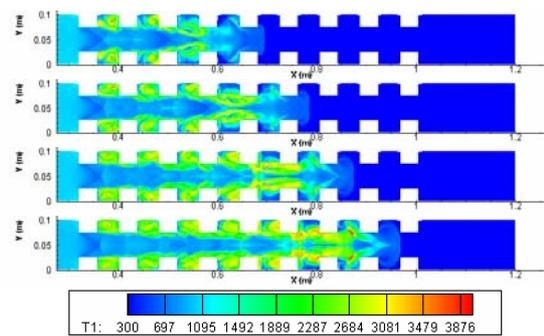
**Fig. 4:** Snapshots of temperature fields in the channel with regular orifice plates. The upper snapshot corresponds to  $480 \mu\text{s}$ . Other snapshots are plotted with the time interval of  $100 \mu\text{s}$
