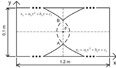
**Fig. 1:** Schematic of shaped parabolic obstacles in the 2D channel
