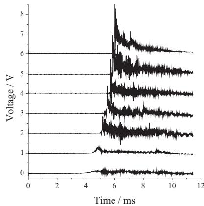
**Fig. 7:** Pressure records in the run with igniter energy of 5 J.
