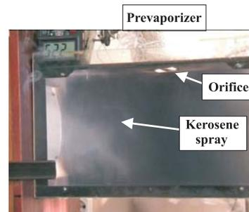
**Fig. 3:** Visualization of kerosene spray exhasting from the prevaporizer orifice (top) at prevaporizer wall temperature of 225 °C.
