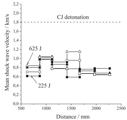
**Fig. 6:** Measured mean shock wave velocities as a function of distance from the igniter in 4 runs with the ignition energy varied from 225 to 625 J.
