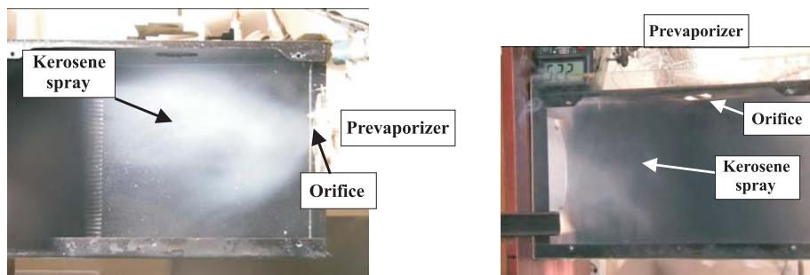
**Fig. 2:** Visualization of kerosene spray exhausting from the prevaporizer orifice (left) at prevaporizer wall temperature of 90 °C.
