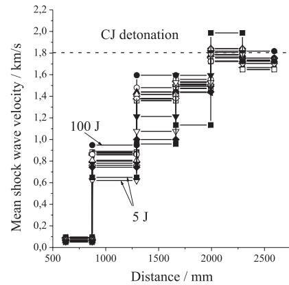
**Fig. 8:** Measured mean shock wave velocities as a function of distance from the igniter in 12 runs with the ignition energy varied from 5 to 130 J.
