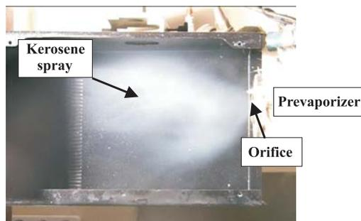
**Fig. 2:** Visualization of kerosene spray exhasting from the prevaporizer orifice (left) at prevaporizer wall temperature of 90 °C.
