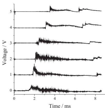
**Fig. 5:** Pressure records in the run with igniter energy of 225 J.
