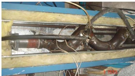
**Fig. 4:** The curved tube segment in the thermostat.
