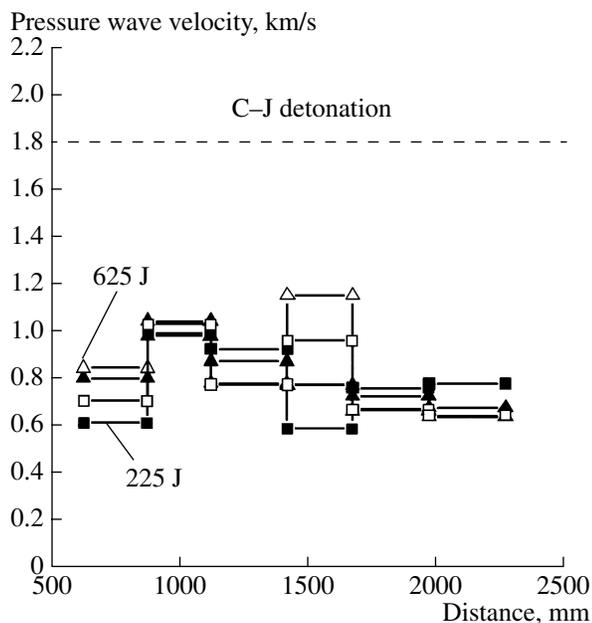
**Fig. 2.** Change in the pressure wave velocity in a kerosene-air flow in four runs in the straight detonation tube at an ignition energy from 225 to 625 J.
