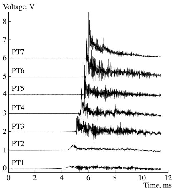
Fig. 4. Records of pressure transducers PT1–PT7 for the DDT in the run with the ignition energy 5 J.
