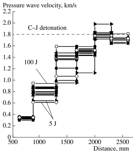
**Fig. 3.** Change in the pressure wave velocity in a kerosene-air flow in 12 runs in the detonation tube with the Schelkin spiral and the coil at an ignition energy from 5 to 100 J.
