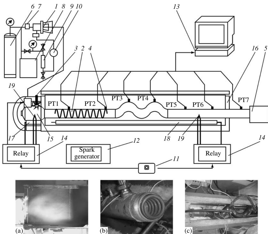
Fig. 1. Scheme of the experimental setup with (a) a kerosene prevaporizer, (b) a Shchelkin spiral, and (c) a tube coil.
