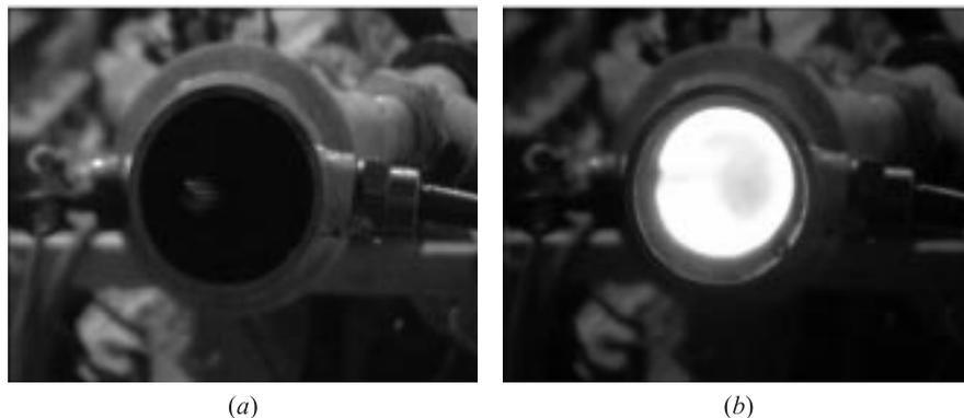
**Figure 2** Preheating the main tube during the starting procedure: (a) start-up spark plug triggering, and (b) onset of a two-phase diffusion flame
