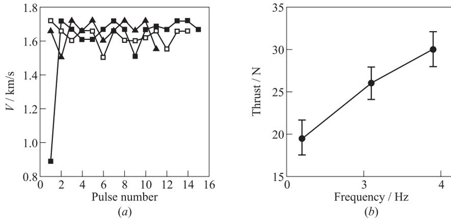
**Figure 3** (a) Multipulse operation of the PDE demonstrator at the operation frequency of 3.9 Hz. Symbols show pulse-to-pulse variation of the mean velocity of the pressure wave at the measuring segment PT4–PT5 in the main tube for three independent runs. Total ignition energy per pulse is 30 J
