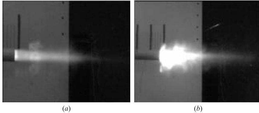
**Figure 4** Pulse detonation engine nozzle plume produced by detonation (*a*) and deflagration (*b*)
